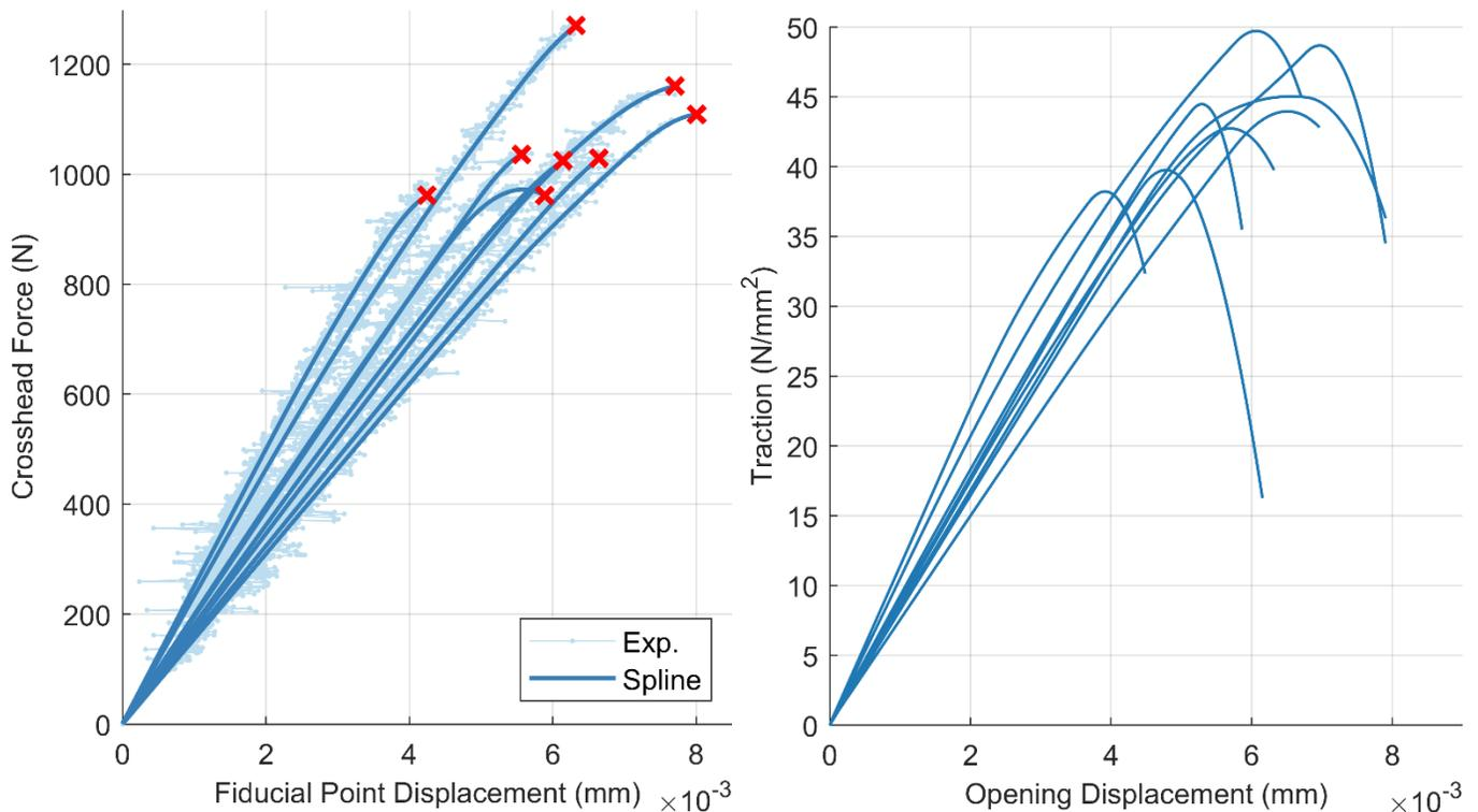
Figure 3. (a) Measured force-displacement responses ( $n=7$ ) overlaid with smoothing spline. Red markers indicate the point of rapid crack growth. (b) Traction-separation responses extracted from smoothing splines using the method of Watson et al. [7]
