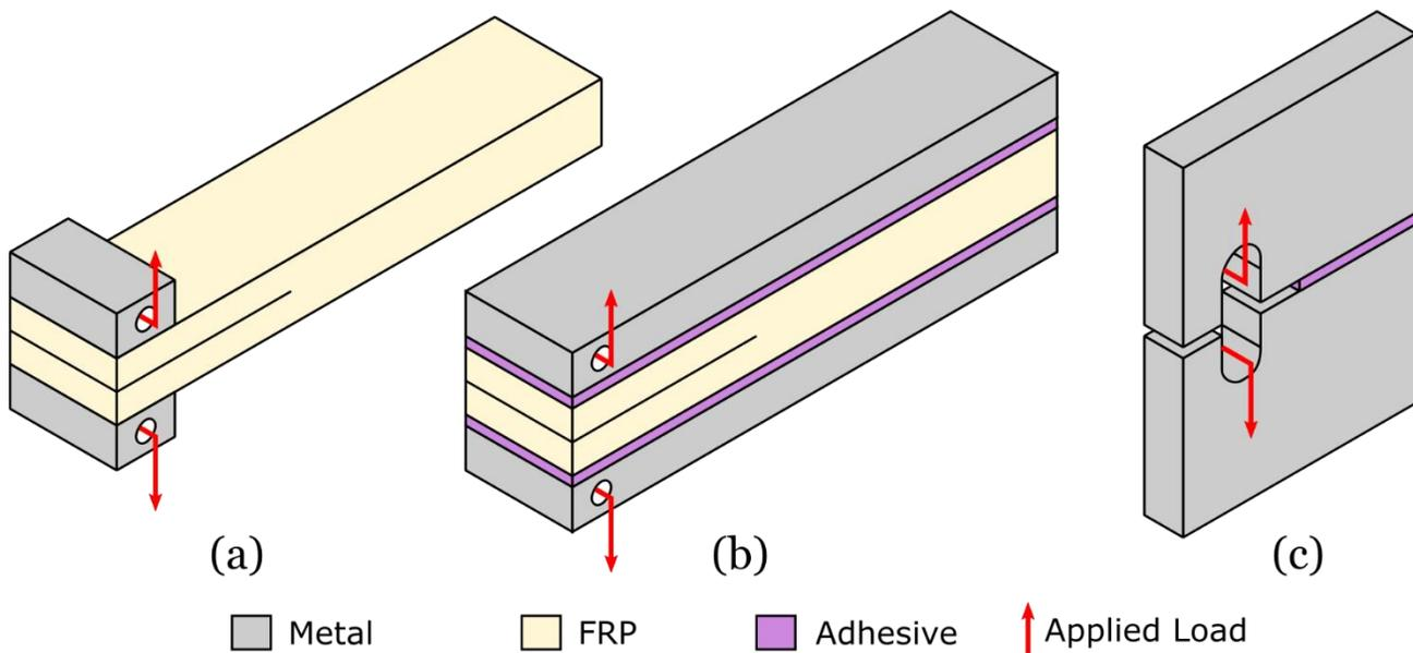
Figure 1. (a) A standardized DCB specimen, (b) a reinforced DCB specimen [6] (c) Watson RDCB for adhesives [7]. Specimens are not to scale.
