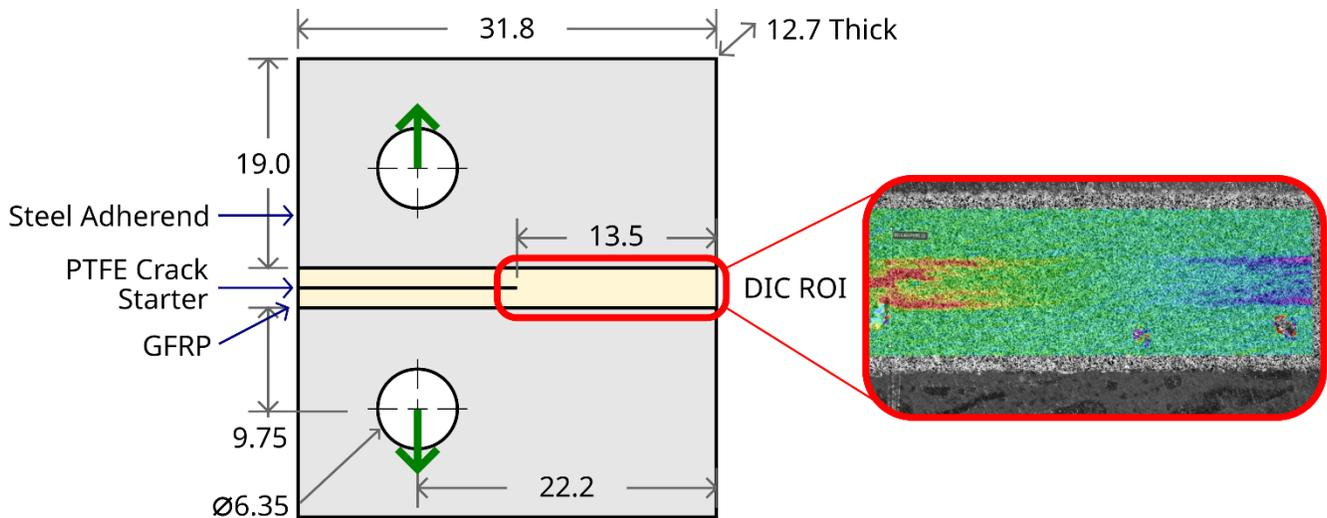
Figure 2. cRDCB schematic and dimensions. Green arrows represent load application via pins, while the red box and right image show DIC region of interest and example strain contours.
