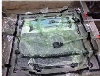
Figure 1. Seemann Composite Resin Infused Molding Process
