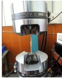
Figure 7 Tensile shear test
