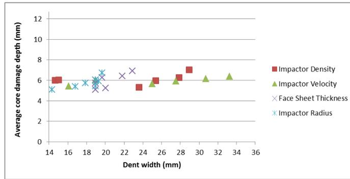
Figure 9: Average core damage depth versus dent width, for the studies varying the impactor and the skin thickness.
