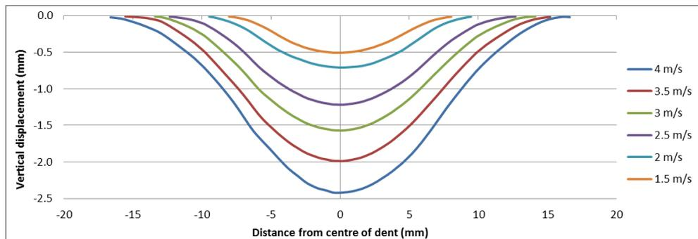
Figure 3: Dent profiles for different impactor velocities
