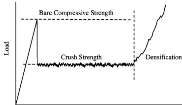
Figure 7: Typical Honeycomb Core Crush Curve [6]
