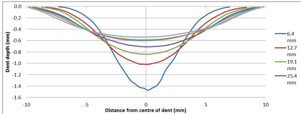
Figure 4: Dent profiles for different impactor radii, at constant energy levels
