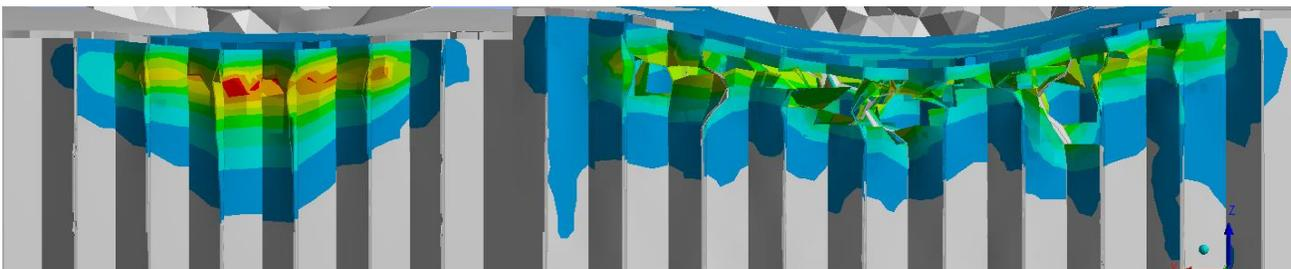
Figure 6: Side by side comparison of shape of damage region for low energy (0.6 J; left) and high energy (4.3 J; right) impact from the velocity study, coloured region indicating yielding.
