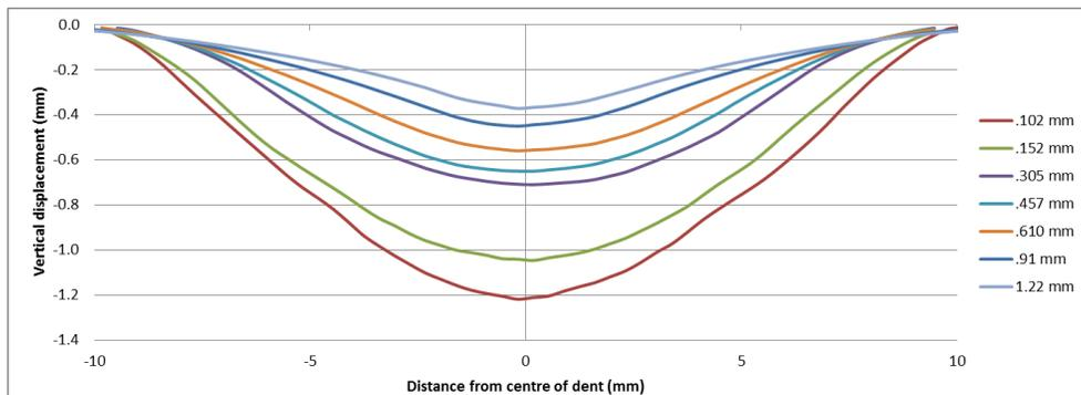
Figure 5: Dent profiles for different face sheet thicknesses, at constant energy levels
