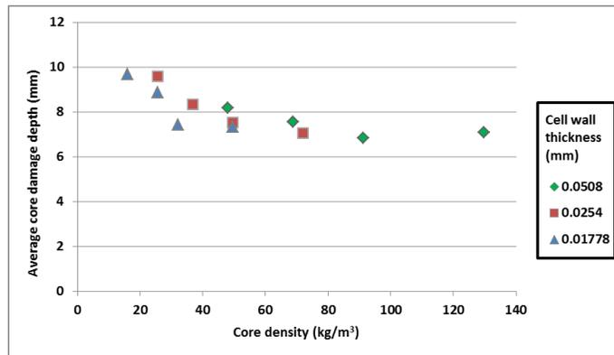
Figure 10: Average core damage depth versus core density, for core density study
