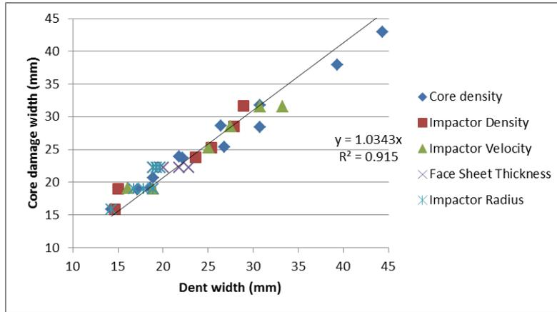
Figure 7: Core damage width versus dent width for all studies
