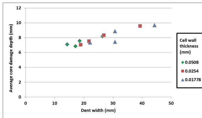
Figure 6: Average core damage depth versus dent width, for core density study
