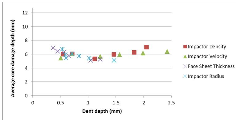
Figure 8: Average core damage depth versus dent depth, for the studies varying the impactor and the skin thickness.
