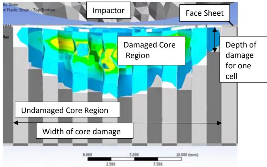
Figure 2: Core damage measurement, with coloured region indicating yielding.
