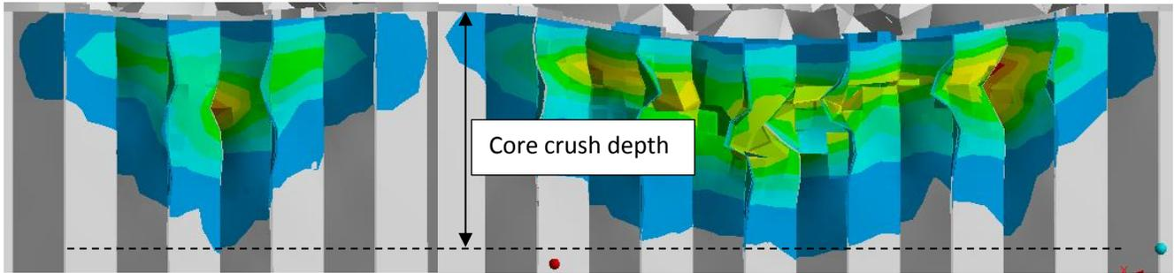
Figure 8: Depth of core damage region, immediately after impact (left) and at point of maximum displacement of impactor (right)
