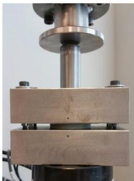
**Figure 2: Shear punch tool (ASTM D732) and setup**
