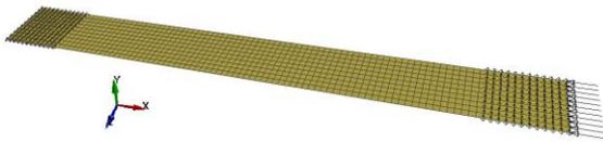
Figure 1: The FE mesh, boundary conditions and applied load.
