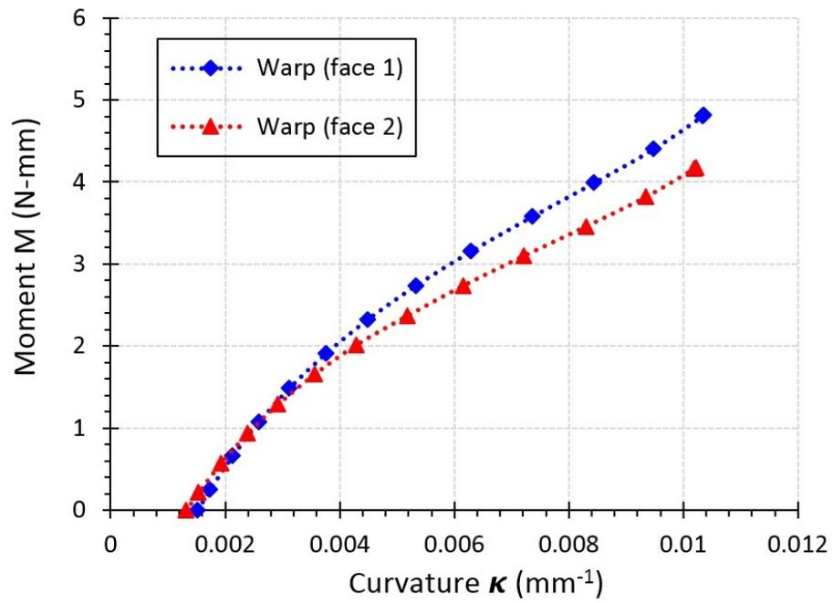
Figure 3. Bending moment versus curvature of 5HS prepreg sample in warp direction at room temperature.
