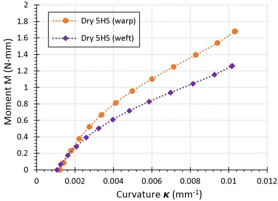
Figure 5. The difference between warp and weft directions in dry 5HS.
