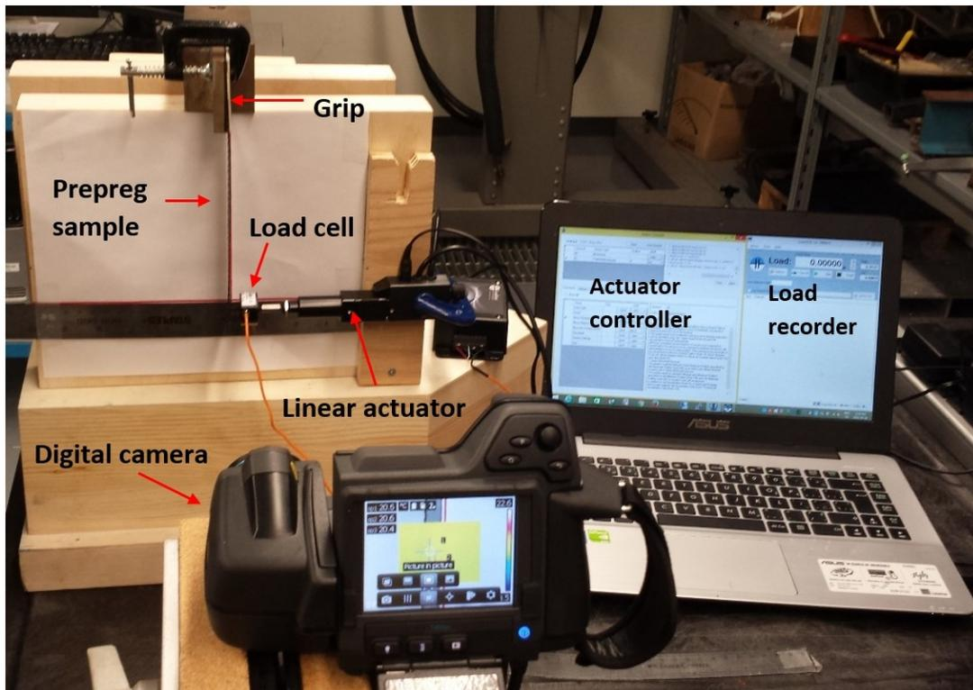
Figure 1. Bending test setup for prepreg characterization purposes.
