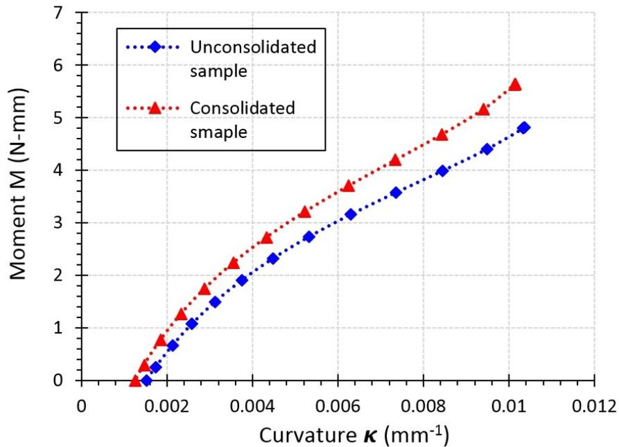
Figure 7. Bending moment versus curvature for consolidated and unconsolidated samples (warp-face 1).
