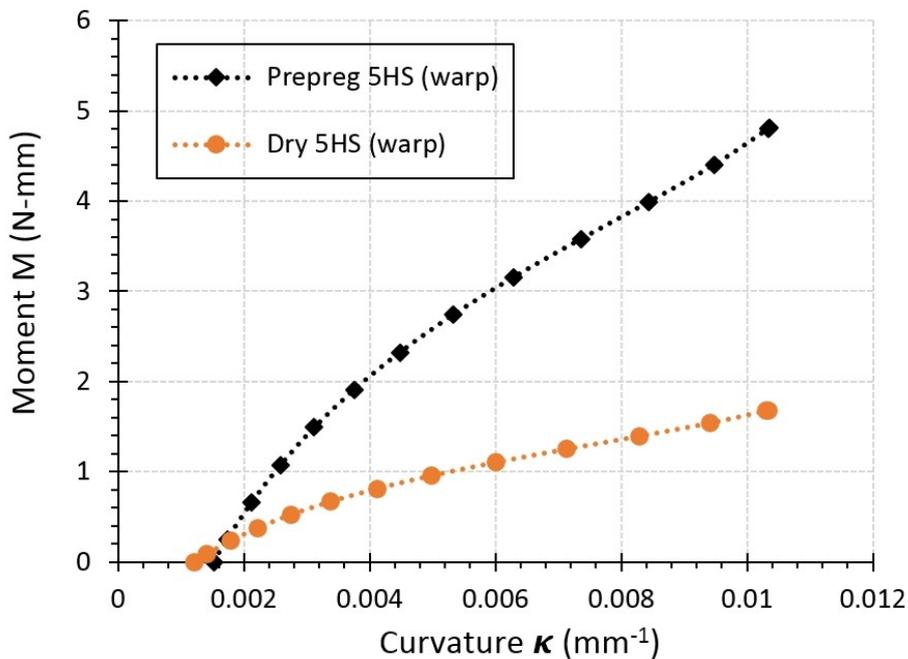
Figure 6. The difference between prepreg and dry samples in warp direction.
