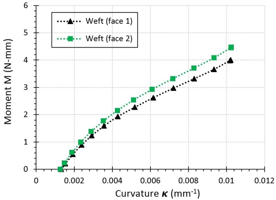
Figure 4. Bending moment versus curvature of 5HS prepreg sample in weft direction at room temperature.
