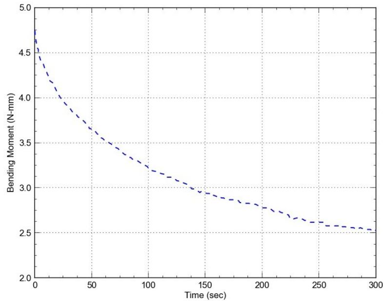
Figure 8. Relaxation of 5HS prepreg sample (warp) recorded at room temperature.
