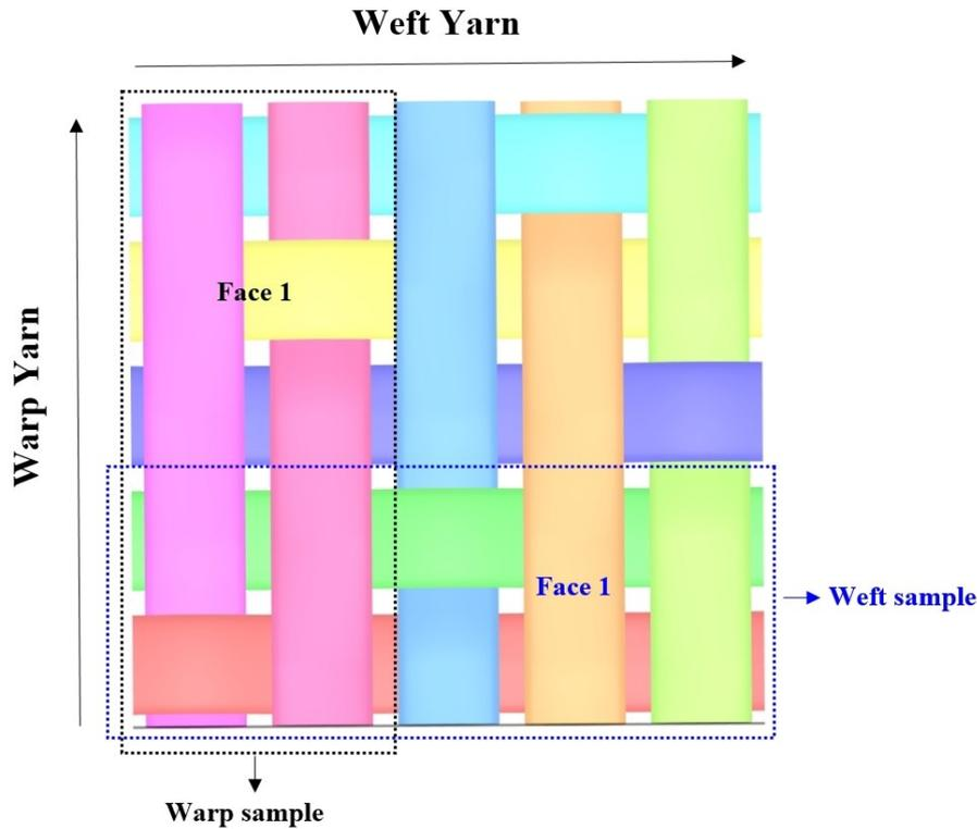
Figure 2. 5HS prepreg samples and yarn direction to the applied load.
