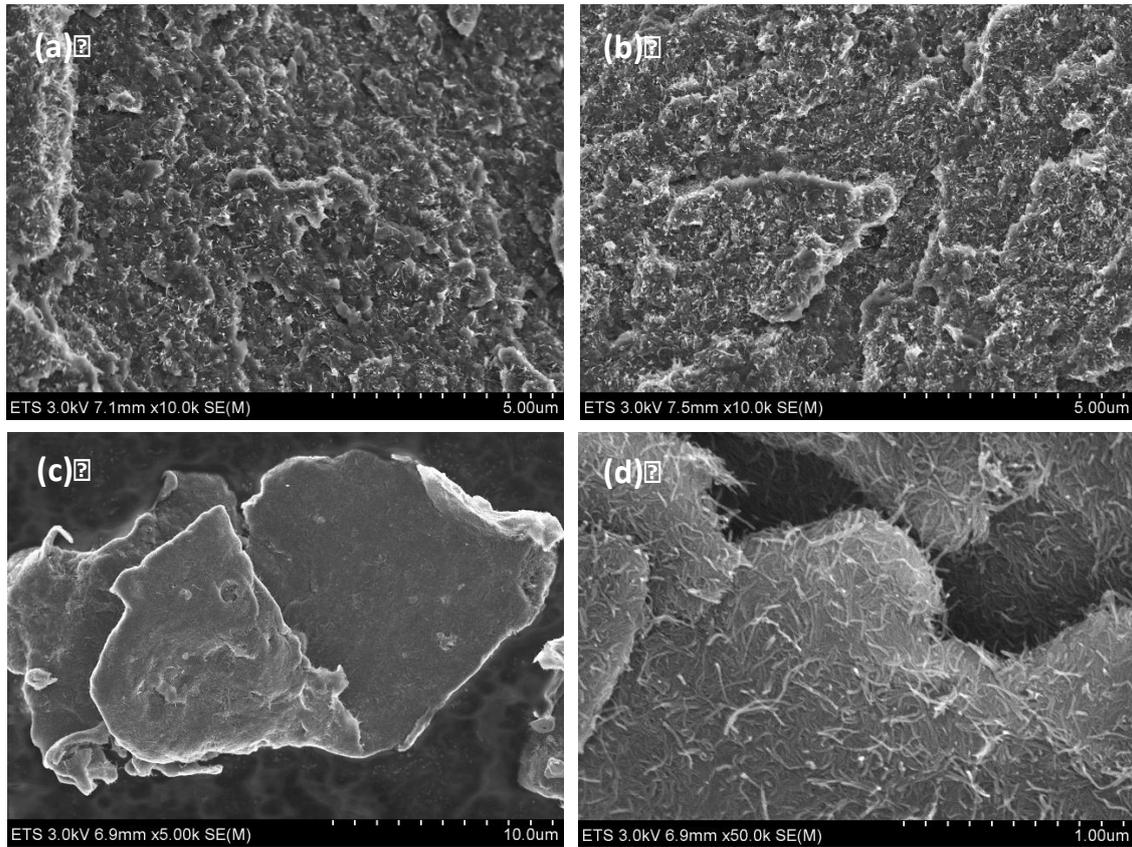
Figure 3: SEM micrographs of (a) nanocomposites containing 5 wt.% MWCNTs and (b) nanocomposite containing 15 wt.% MWCNTs, both prepared using the micro-extruder, (c) a ball-mill mixed nanocomposite pellet (i.e., cluster) with nanotube concentration of 15 wt.% and (d) a higher magnification image of (c).
