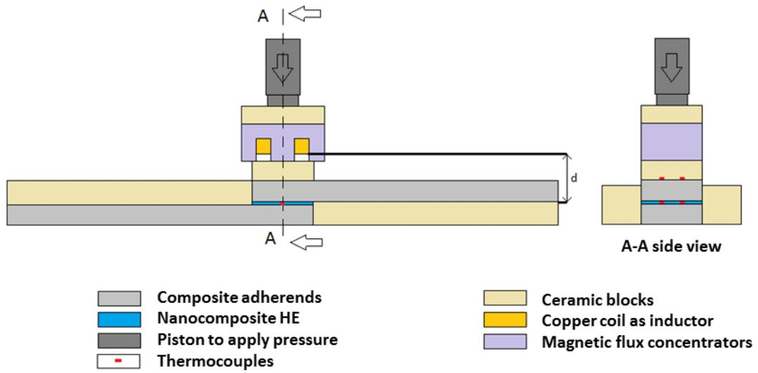
Figure 1: Schematic representation of the induction welding setup.
