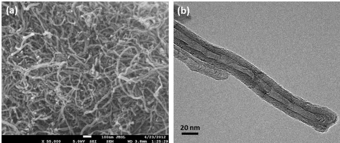
Figure 2: SEM (a) and TEM (b) micrographs of MWCNTs used in this study.
