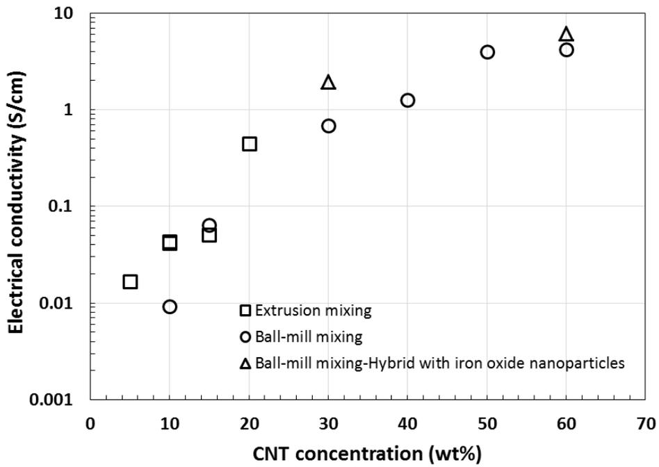
Figure 4: Electrical conductivity of the nanocomposite HEs as a function of MWCNT concentration. The hybrid nanocomposites contain 37 wt.% (for the left point) and 10 wt.% (for the left point), respectively.
