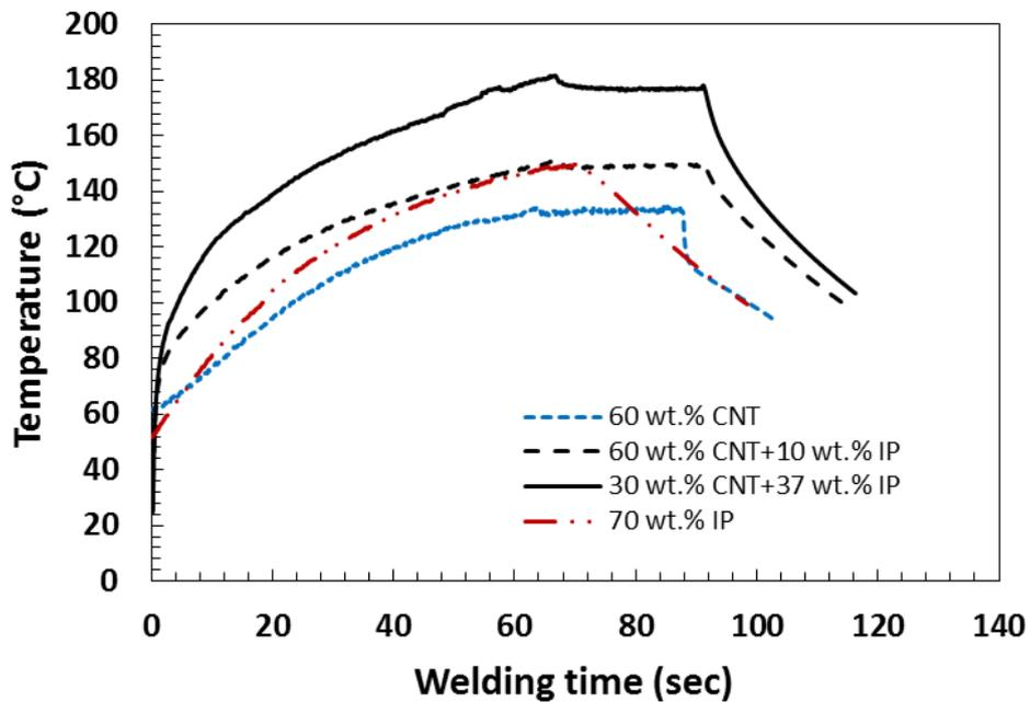
Figure 5: Heating behavior of the fabricated nanocomposite HEs as temperature variation at the weld interface as a function of welding time at the input current of 700A.
