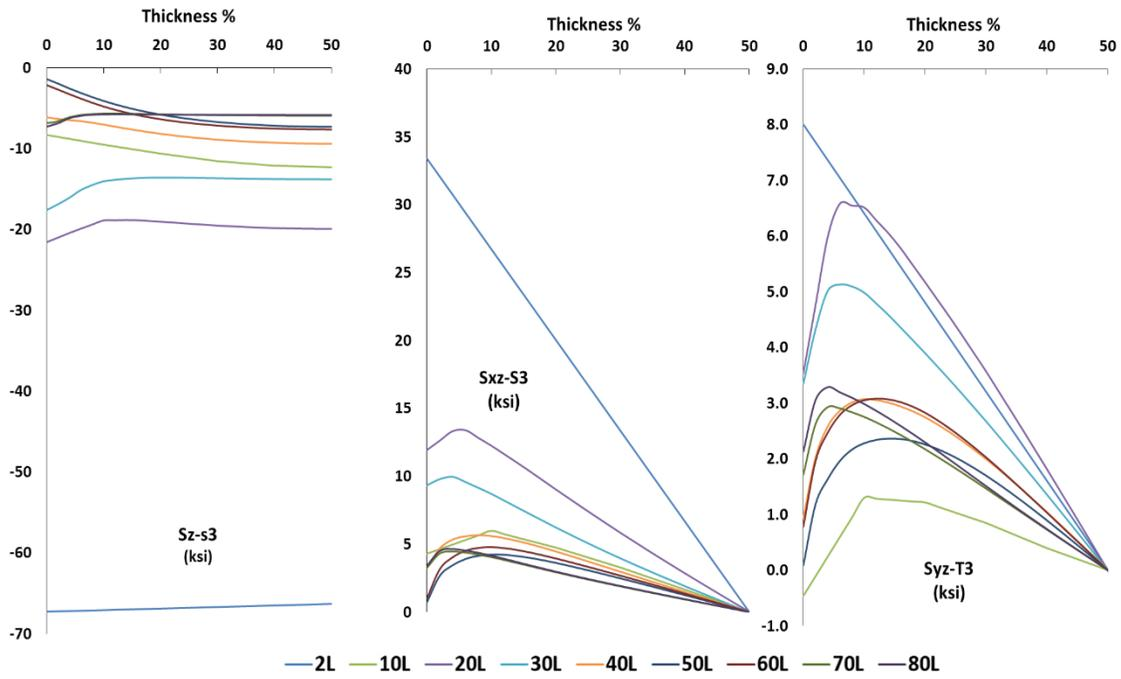
Figure 6: Interlaminar stresses distributions along the thickness at outer edge of the washer
