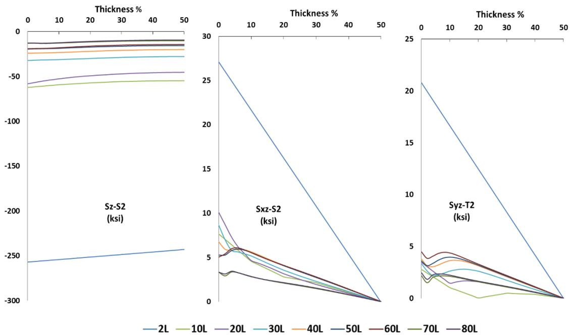
Figure 5: Interlaminar stresses distributions along the thickness between inner at outer edge of the washer
