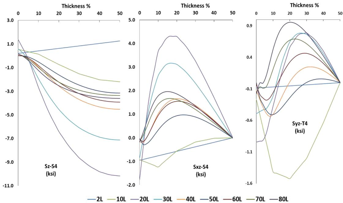
Figure 7: Interlaminar stresses distributions along the thickness at radial distance of  $1.25 \times$  hole diameter
