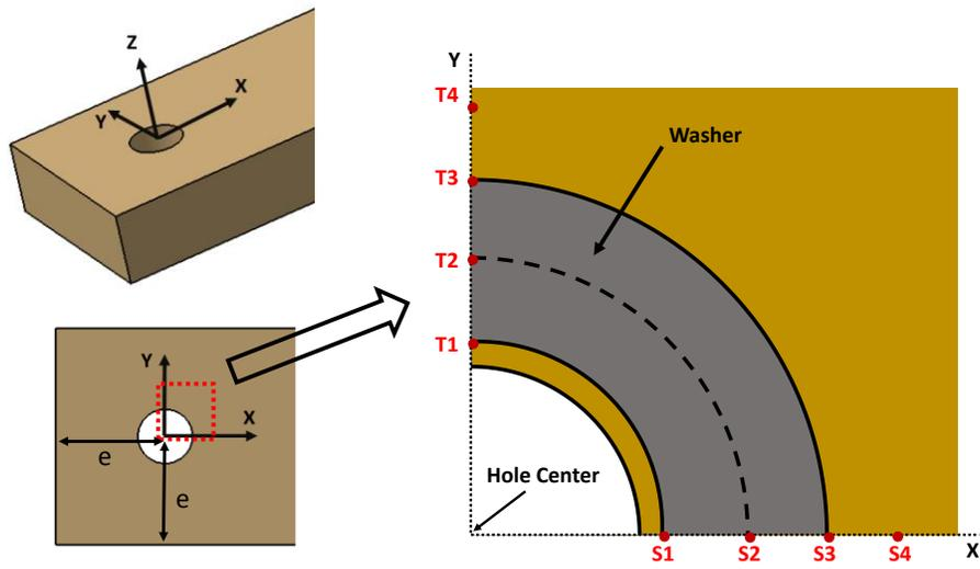
Figure 3: Defined coordinate system and selected points position
