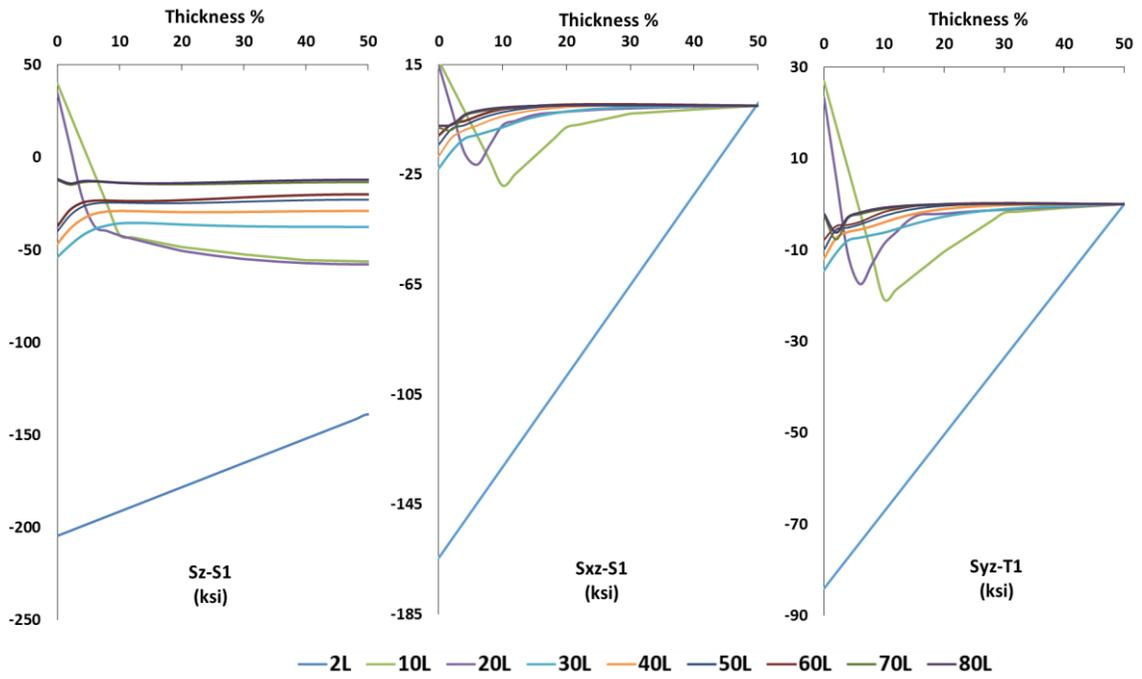
Figure 4: Interlaminar stresses distributions along the thickness at the inner edge of the washer
