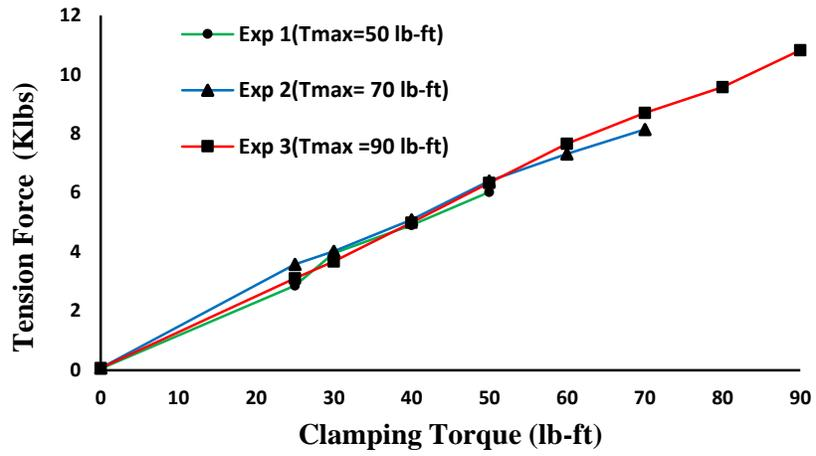
Figure 2: Tension force at bolt shaft vs clamping torque\
