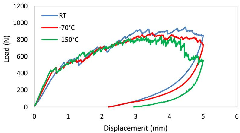
Figure 6. Load-displacement curve for the 12.7 mm diameter indenter.
