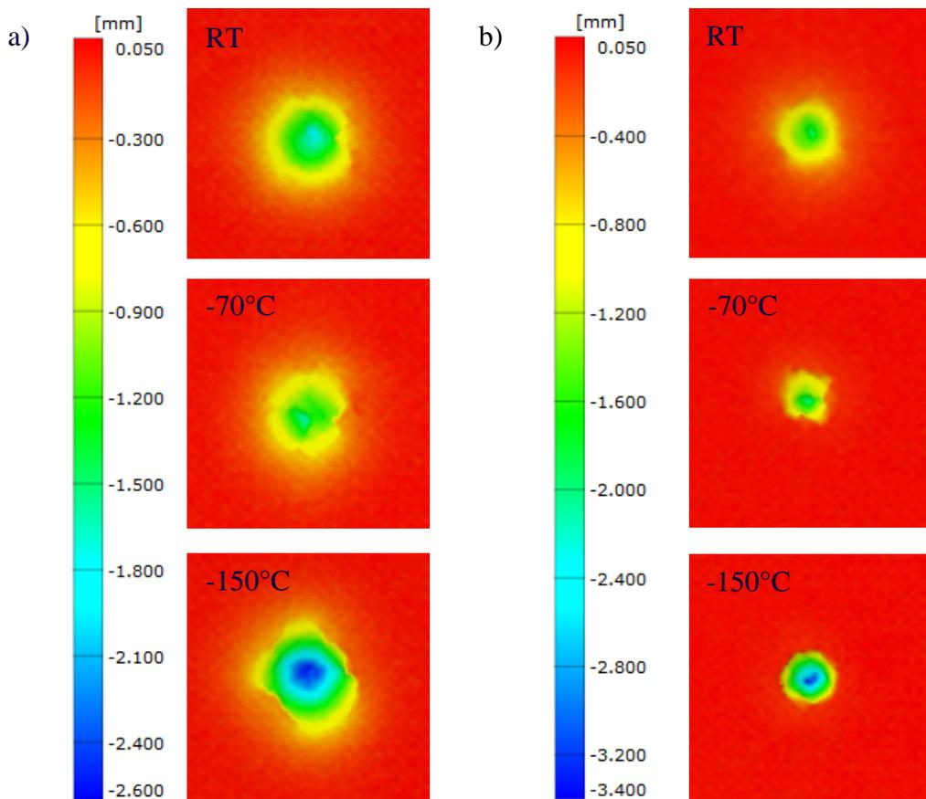
Figure 7. Residual depth of indentation for a) the 25.4 mm diameter and b) 12.7 mm diameter indentors.
