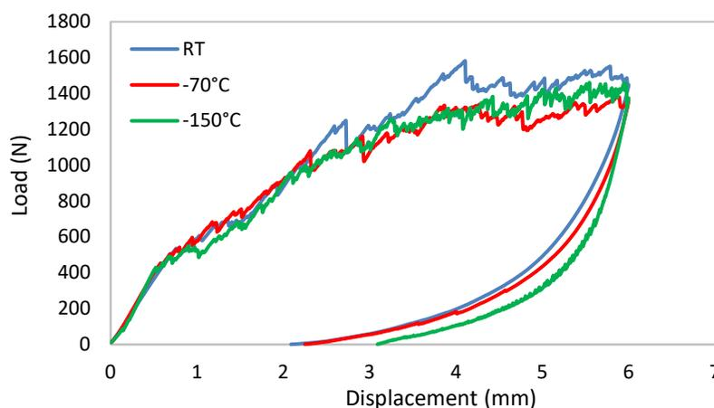
Figure 5. Load-displacement curve for the 25.4 mm diameter indenter.
