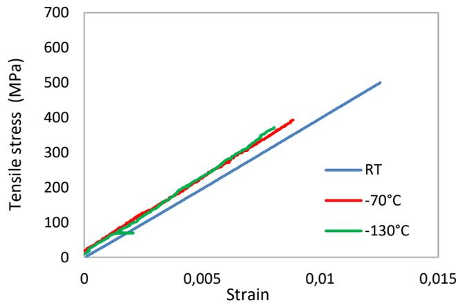
Figure 3. Stress-Strain curves for the [(+45/-45)/(0/90)/(0/90)/(+45/-45)]<sub>s</sub> laminate in the 0°- direction.
