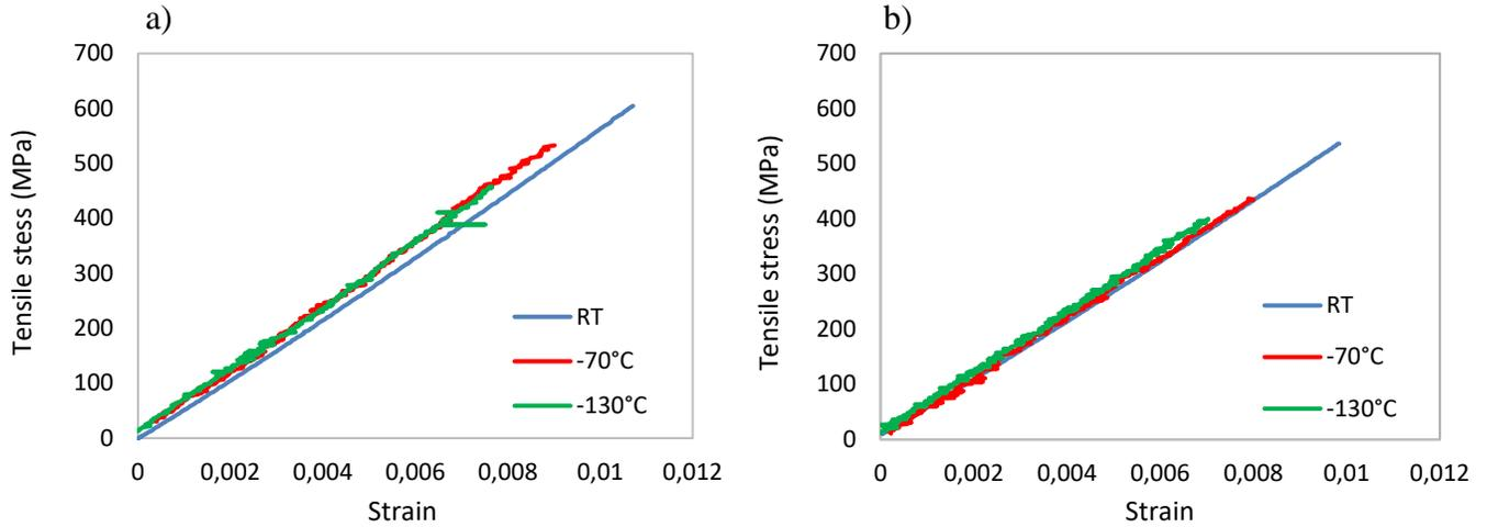
Figure 2. Stress-strain curves for the [(0/90)<sub>5</sub>] laminate in the a) 0°- direction and b) 90°- direction.
