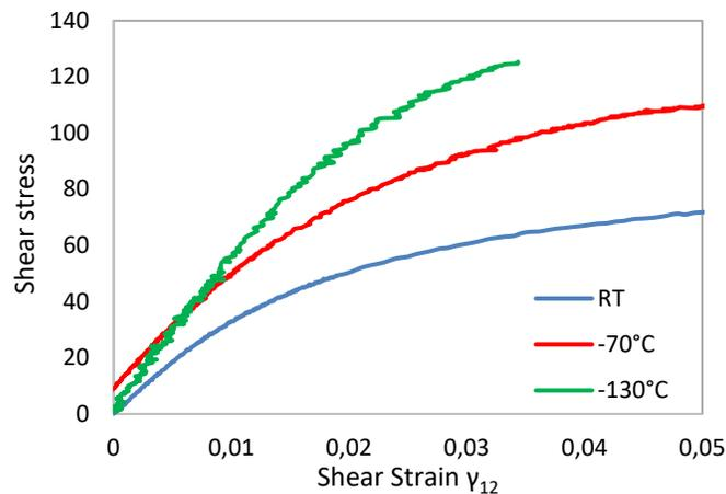
Figure 4. Shear stress-strain curves at room temperature,  $-70^{\circ}\text{C}$  and  $-130^{\circ}\text{C}$ .
