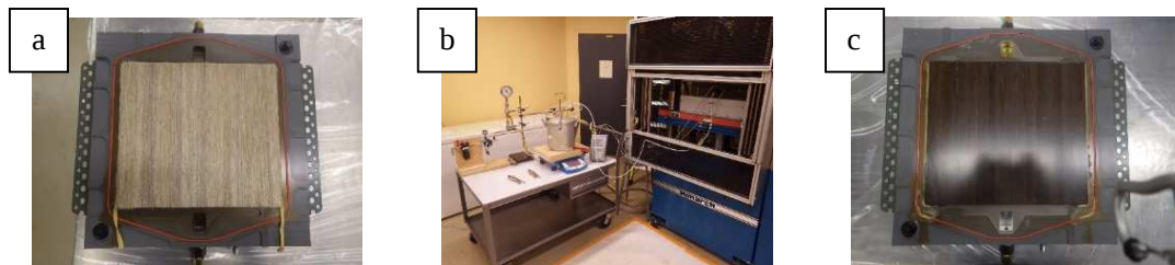
Figure 1. Plaques processing: a) plies stacking b) VARTM setup c) Molded plaque
