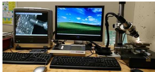
Figure 7. Roughness measurement setup
