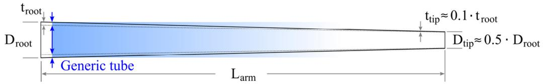
Figure 2. Overall dimensions of the composite cross arm and the generic composite tube cross section properties.
