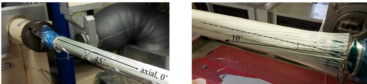
Figure 4. Fibre layup in  $0^\circ$  and  $45^\circ$  (left) as well as in  $10^\circ$  (right) by filament winding
