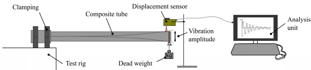
Figure 7. Free decay test setup for analysing the damping performance of the different cross section configurations of the generic composite tubes
