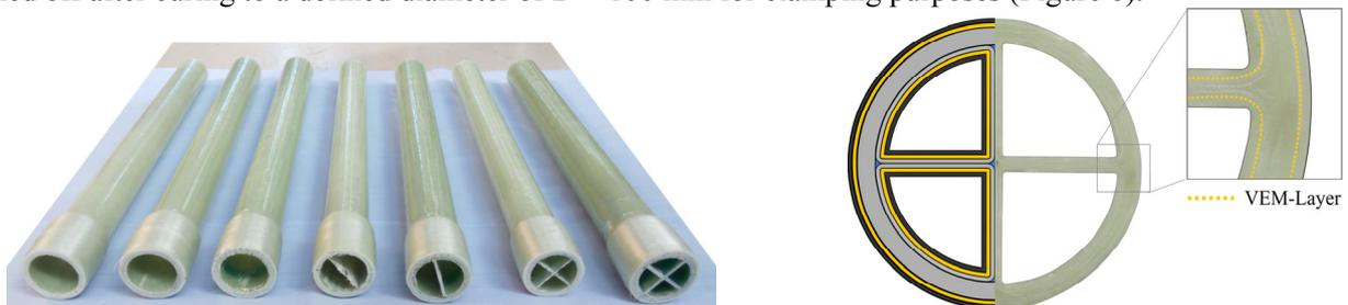
Figure 6. Manufactured GFRP tubes (left); Grinding pattern of the generic composite tube concept (i) (right)
