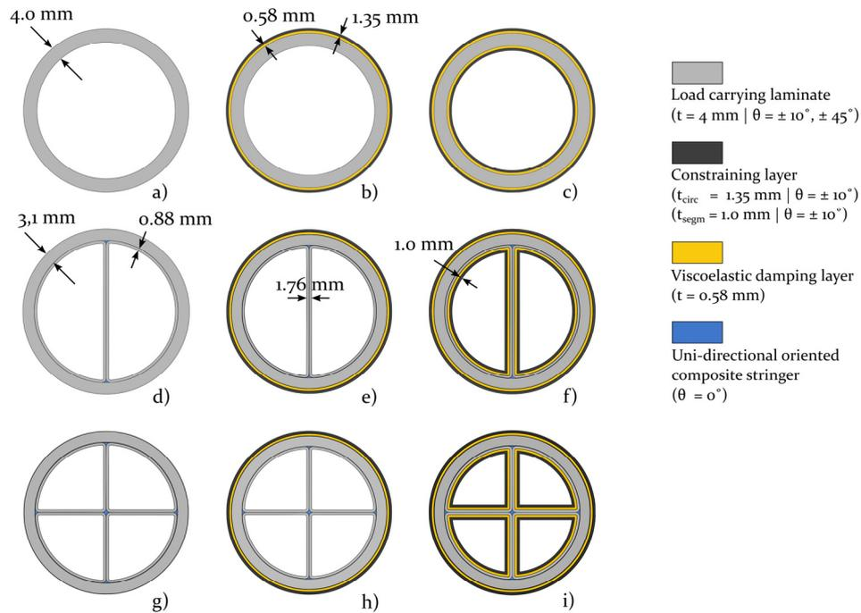
Figure 3. Overview of the various cross sectional concepts of the generic composite tube with different locations of the viscoelastic damping layers
