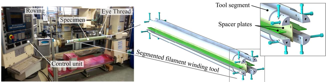
Figure 5. Manufacturing of the generic tubular structure using a filament winding machine
