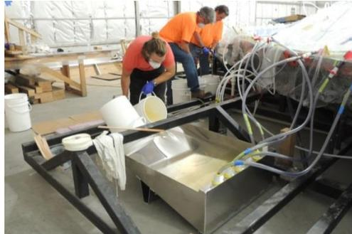
Figure 8: Resin feed tray and mixing station (one of 4).
