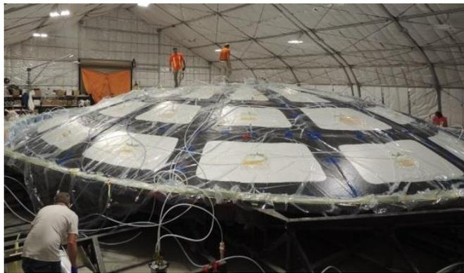
Figure 1: Vacuum infusion of a 15 metre radio telescope, just 12 minutes into a 2 hour infusion.
