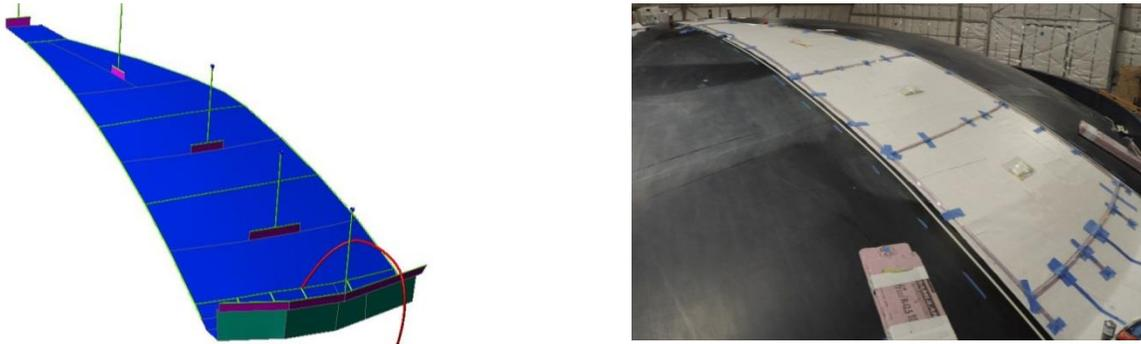
Figure 6: Large scale test part on primary reflector mold. LHS flow model, RHS test part setup.
