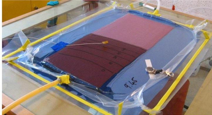
Figure 5: A typical permeability test panel setup.
