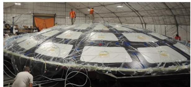
Figure 9: Full dish infusion at 12 minutes, LHS, model, RHS actual part.
