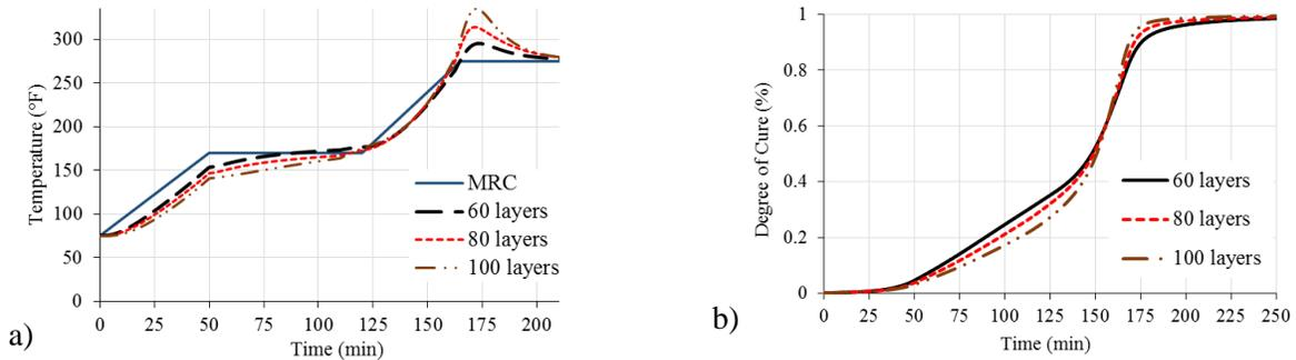
Figure 4 The comparison of the centerline a) temperature b) cure profiles from simulation.
