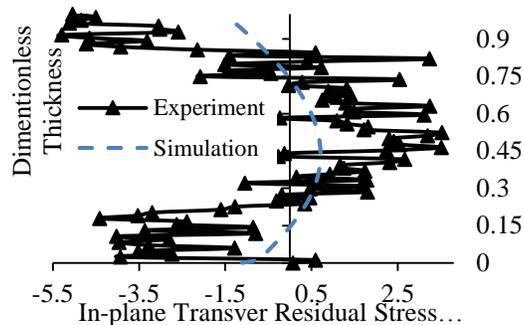
Figure 10 Comparison of in-plane transverse residual stress in unidirectional laminate plate,  $[0]_{80}$  [14].
