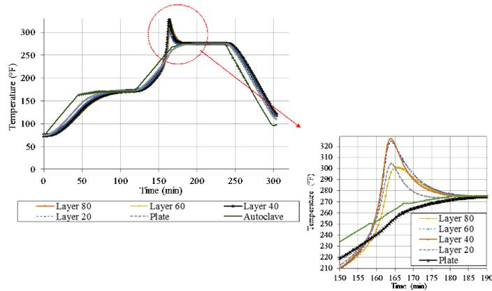
Figure 2 Temperature profile in glass/epoxy laminate from experiment
