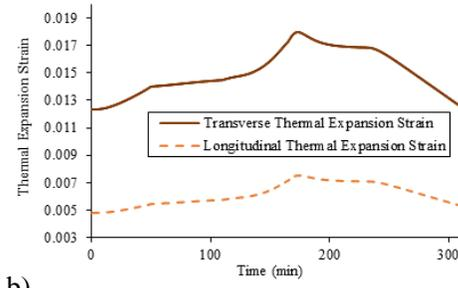
Figure 8 Calculated process stress-free a) transverse shrinkage b) thermal strains in glass/epoxy laminate
