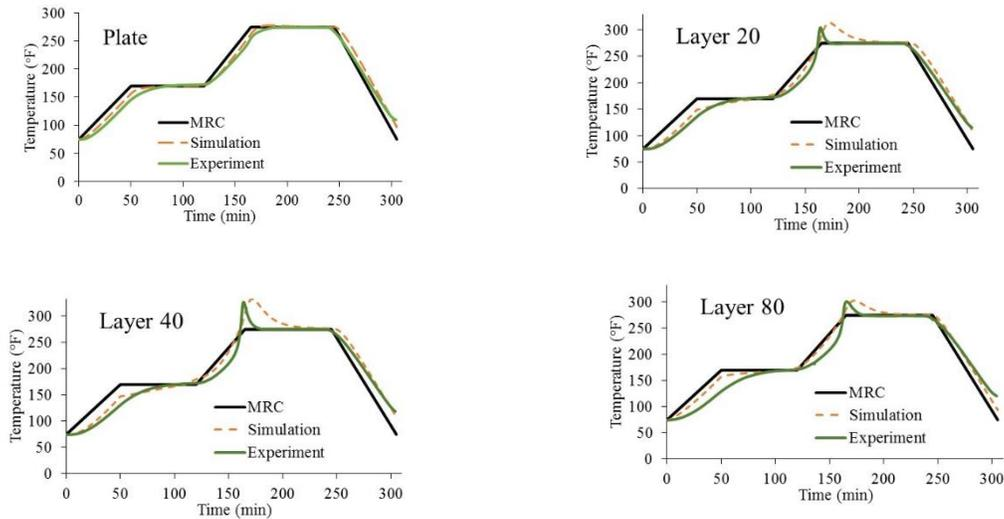
Figure 3 Temperature profiles from experiment and calculated results at different plies.
