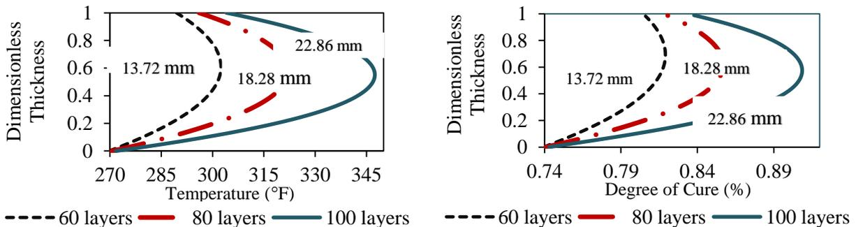
Figure 5 Temperature and cure gradients after 164 min from simulation.
