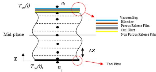
Figure 1 Schematic diagram of the asymmetric boundary conditions.
