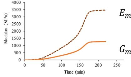
Figure 6 Calculated cure dependent epoxy resin modulus during the curing process
