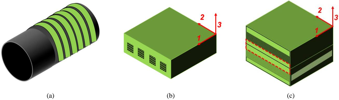
Figure 5. a) Thermoplastic FRPC pipe wound by pre-fabricated fiber reinforced tapes, b) fibers and matrix configuration in fiber reinforced tape and c) fibers and matrix configuration in bonded fiber reinforced tapes
