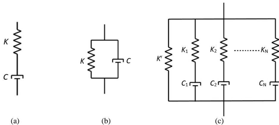
Figure 2. Spring and dashpot element model configurations: (a) Maxwell, (b) Kelvin and (c) generalized Maxwell [7, 9]
