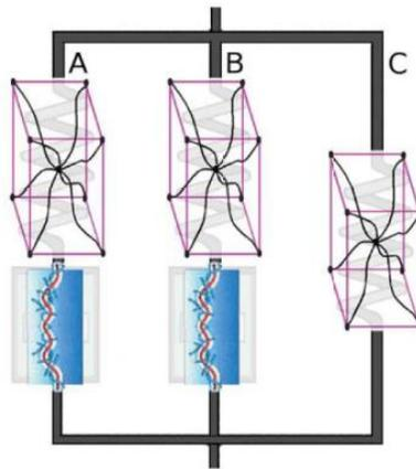
Figure 3. The configuration of elements in Bergstrom-Bischoff three network model [12]
