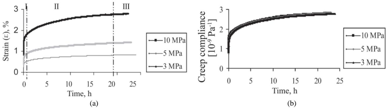
Figure 1. Compressive creep of HDPE for applied stress values of 3, 5 and 10 MPa;
