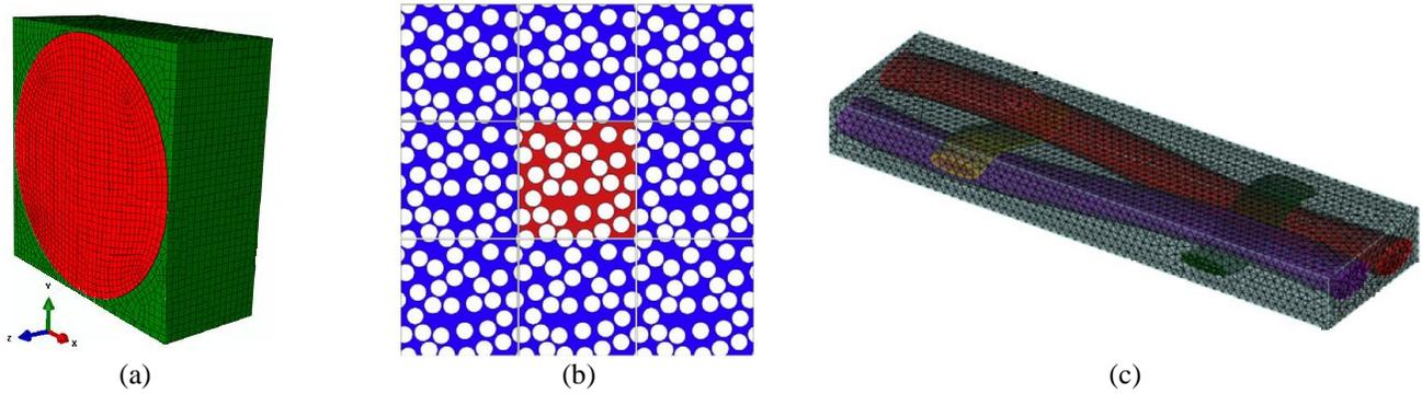
Figure 4. Different RVEs for multi-scale modeling; a) single fiber within the matrix [19], b) a number of fibers distributed by random sequential adsorption algorithm [20] and c) textile composite [21]
