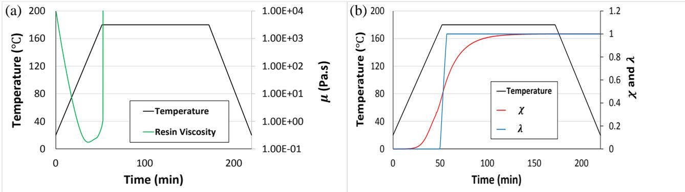
Figure 4. (a) time-history of applied temperature and (b) predicted viscosity, degree of cure, and solidification factor of material
