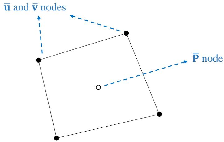
Figure 2. Schematic representation of 4-1 element
