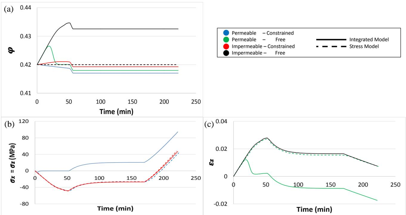
Figure 5. Predicted time-histories of the: (a) resin volume fraction, (b) stresses, and (c) total strain in the vertical direction  $\epsilon_z$
