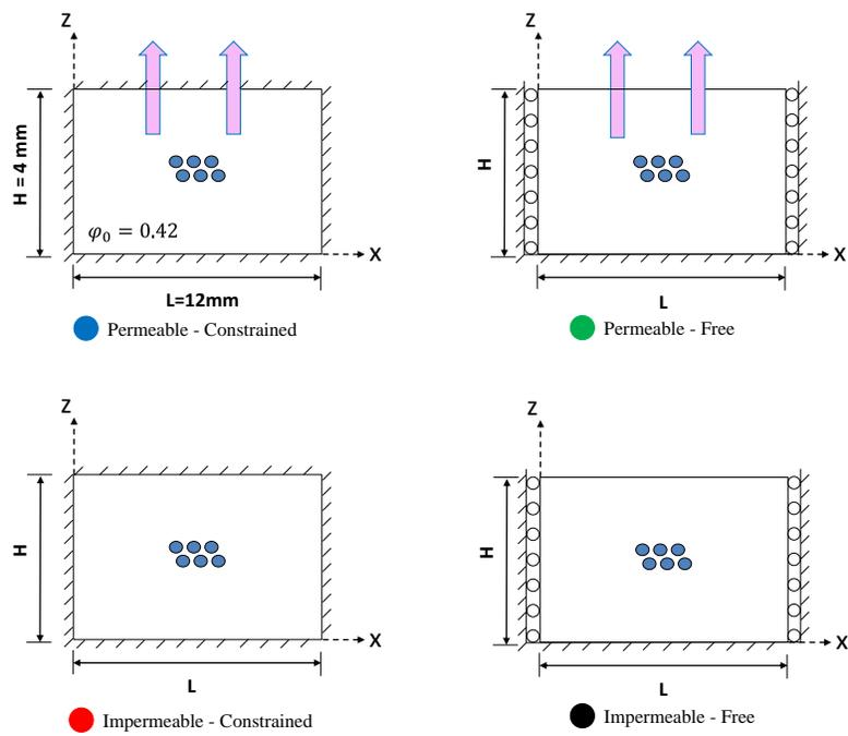
Figure 3. Geometry and different boundary conditions of sample undergoing curing
