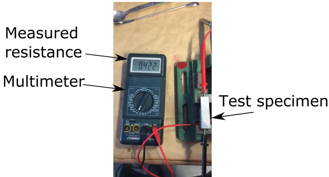
Figure 4: Example preliminary experimental setup to examine the ability to use conductive filament for health monitoring
