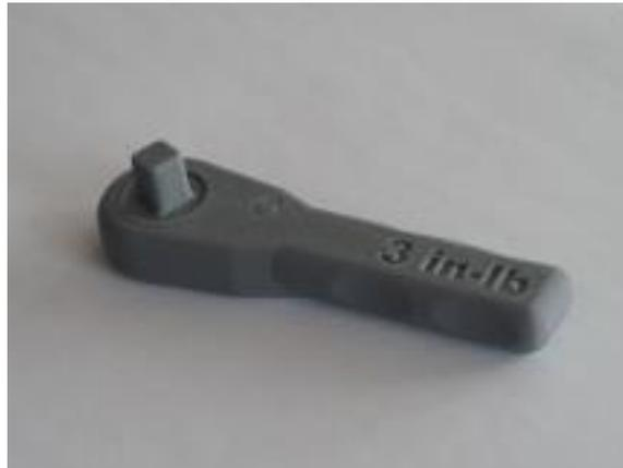
Figure 1: Example functional 3D printed wrench manufactured using a low-cost desktop 3D printer. This wrench was designed for use on the International Space Station [11]. The ratchet wrench demonstrates the ability to create functional components using a FDM manufacturing process.
