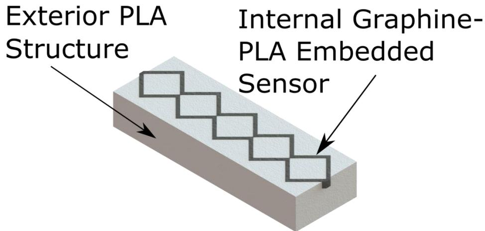
Figure 5: Concept SHM sensor configuration for a FDM printed structure.
