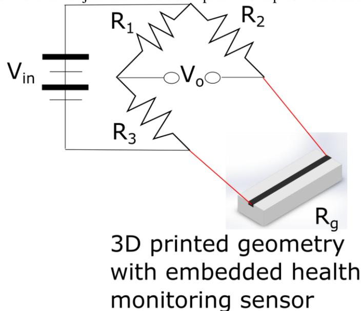
Figure 2: Schematic of a health monitoring sensor embedded within a FDM 3D printed structure
