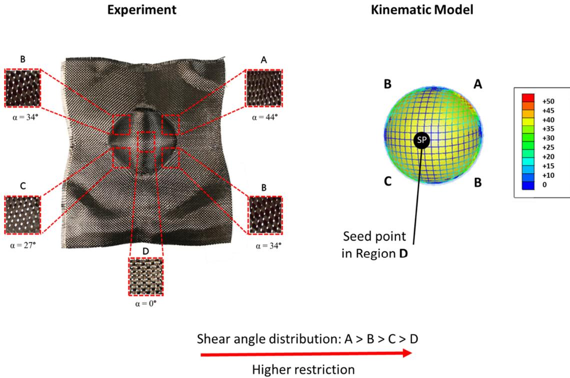
Figure 7. The plain fabric formed onto hemisphere under an asymmetric boundary condition per figure 6. The shear angles are zoomed-in for better visual inspection (left); The kinematic model used the effective seed point approach (right).  $\alpha$  refers to the shear angle of the fabric. The difference between the predicted angles and actual angles was less than 5%.
