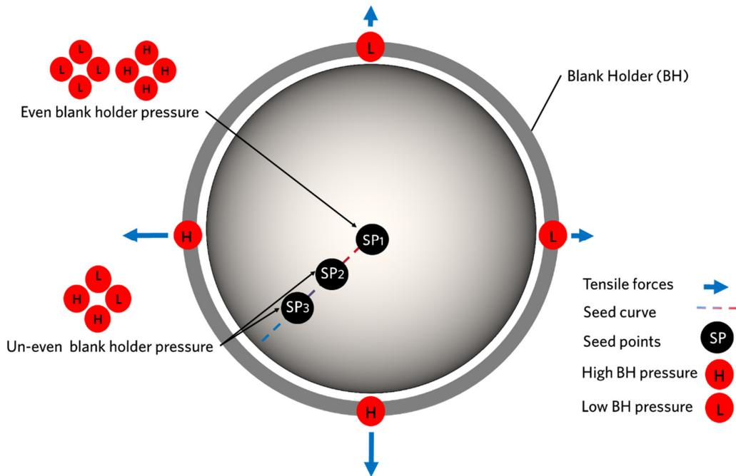
Figure 1. Example of determination of the effective seed point in the kinematic model. SP1 corresponds to the effective seed point when the blank holding pressure is evenly distributed (i.e., all clamps with low or high pressure). When the blank holder pressure distribution is uneven, the seed point can be moved along the resultant force vector shown as dashed line. The blue arrows represent the magnitude of applied force in each blank holder.
