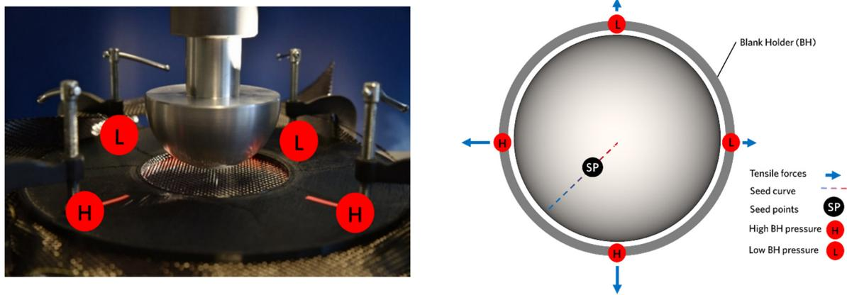
Figure 6. Experimental setup and schematics of boundary condition/pressure distribution in an asymmetric forming trial with discrete blank holders.
