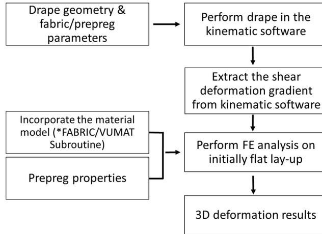
Figure 3. Overview of the hybrid kinematic (HYKE-1) model.
