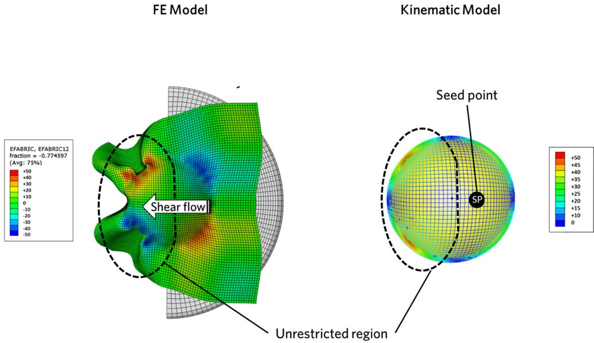
Figure 5. Comparison between the FE-based model and kinematic model for the uneven pressure case (i.e. using half round blank holder).
