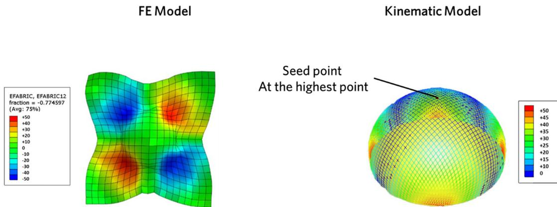
Figure 4. Comparison between the FE-based model and kinematic model for the even pressure case (i.e. using full round blank holder).
