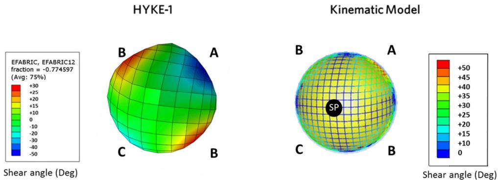
Figure 8. Comparison between the solution obtained using the HYKE-1 model (left) and the kinematic model (right) for the unsymmetrical blank holder condition shown in figures 6 and 7. The difference between the predicted angles by the two models was less than 2%.
