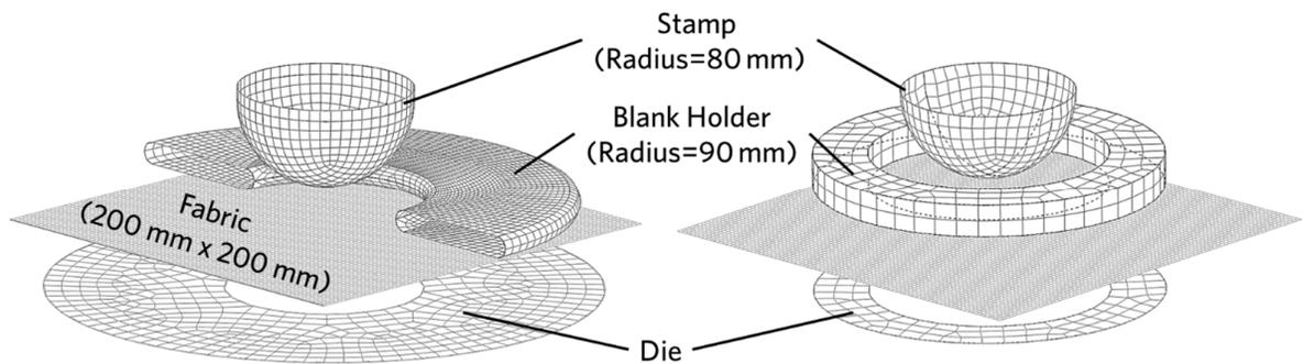
Figure 2. Arrangement of the finite element model for full round (even) and half round (uneven) blank holding conditions.
