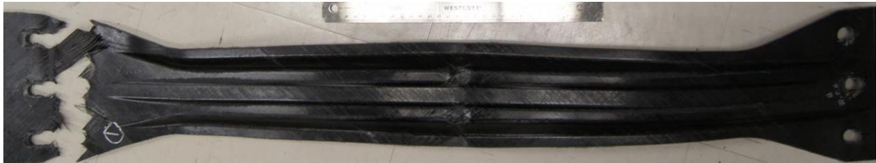
Figure 12: Failure of stamped GF/PP intrusion beam.
