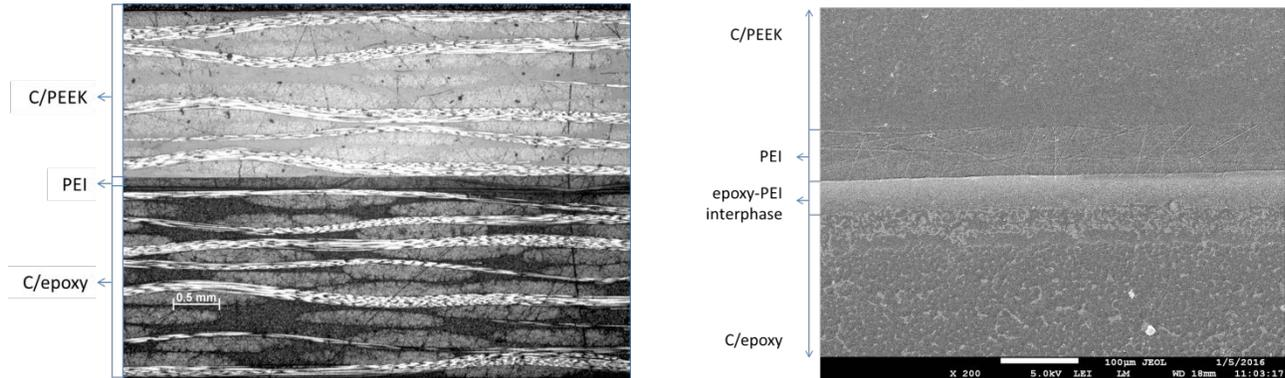
Figure 4. Cross section optical micrograph of etched C/epoxy-PEI-C/PEEK welded sample (left) and SEM detail of the welded joint (right).
