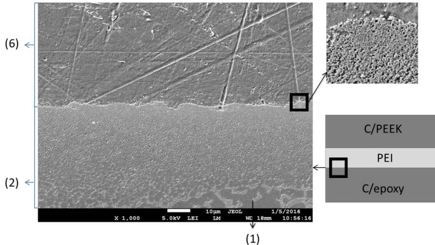
Figure 5. SEM image of post-welded interphase in C/epoxy-PEI-C/PEEK welded sample. Regions (3), (4) and (5) have been displaced by melting and flow of the PEI coupling layer during welding.
