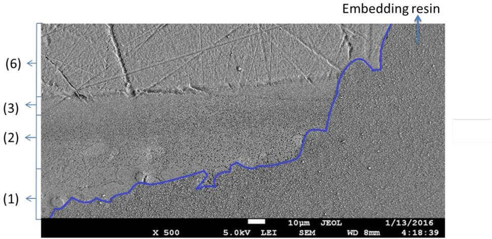
Figure 10. SEM image of a crack path in a C/epoxy-PEI-C/PEEK welded sample (outlined in blue). Numbers in brackets refer to regions in the epoxy-PEI interphase.
