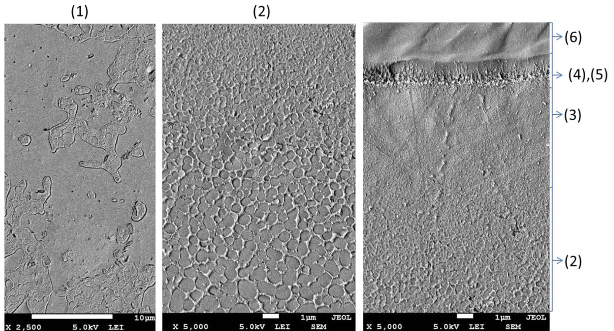
Figure 3. SEM details of different morphologies in epoxy-PEI interphase. Number in between brackets indicate regions within the interphase.
