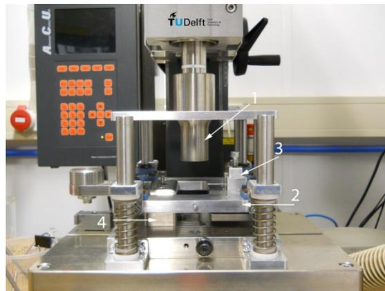
Figure 1. Ultrasonic welding setup: (1) sonotrode, (2) moving platform for top clamp, (3) top clamp, (4) bottom clamp.
