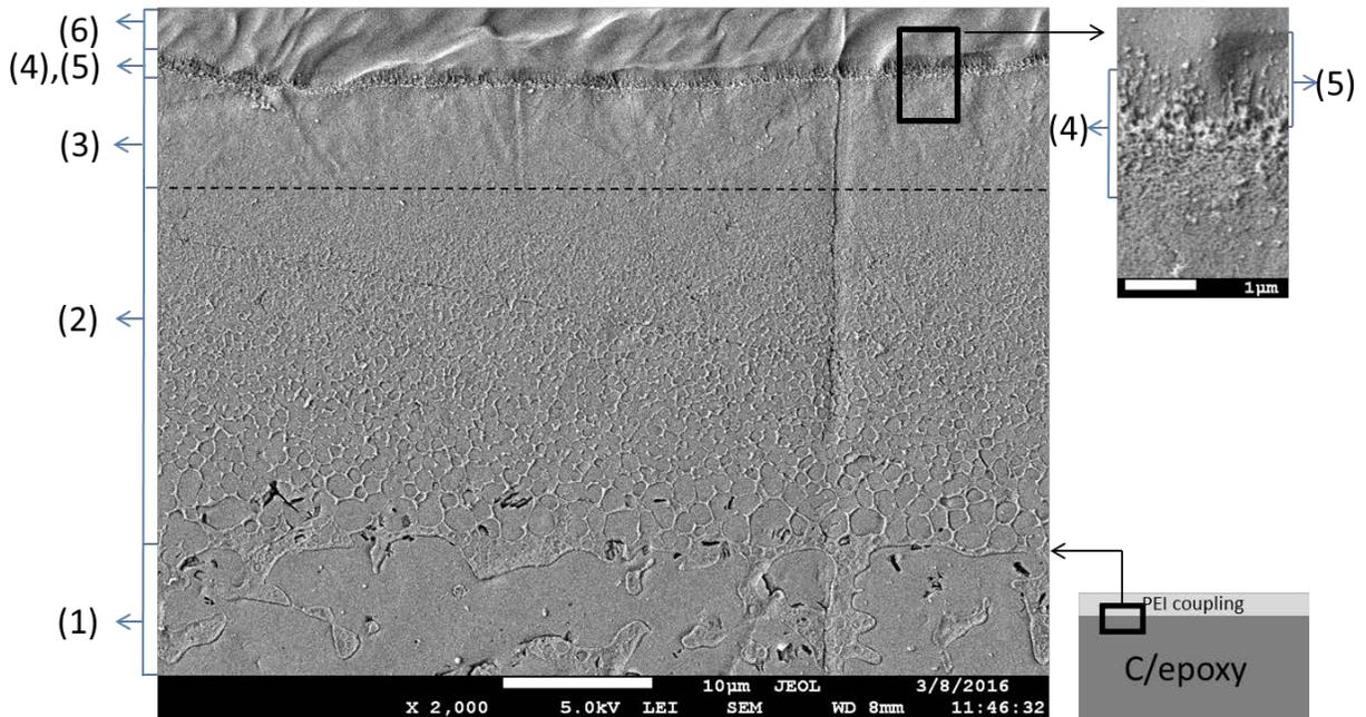
Figure 2. SEM image of the epoxy-PEI interphase. The dotted line indicates approximate location of epoxy-PEI interface prior to co-curing process. Number in between brackets indicate regions within the interphase.
