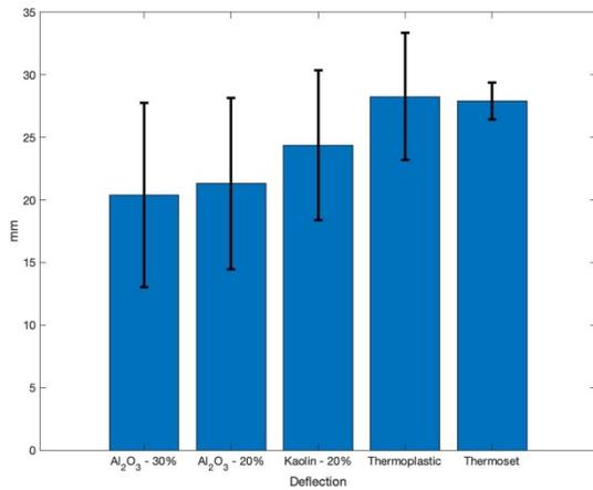
Figure 11: The average range of the maximum deflection value for all 5 experiments
