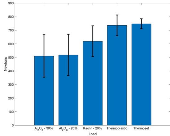
Figure 12: The average range of the maximum deflection value for all 5 experiments
