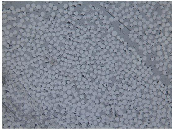
Figure 7: Thermoplastic control rod, no filler
