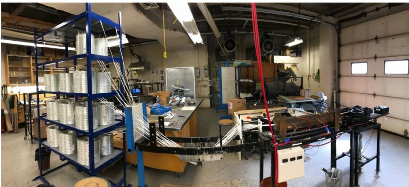
Figure 1: Side view of pultrusion set-up
