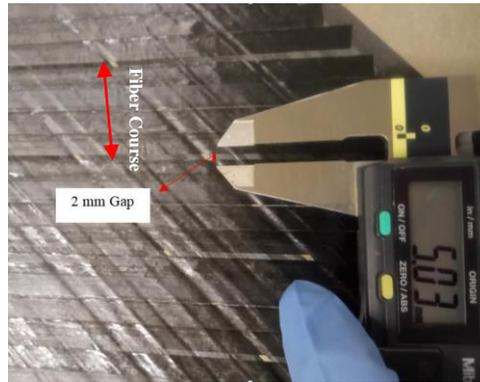
Figure 1: Fiber tows placement including gaps
