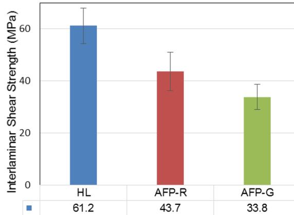
Figure 4: Comparison of the ILSS of the  $[0_2/45_2/90_2/-45_2]_s$  short beam samples
