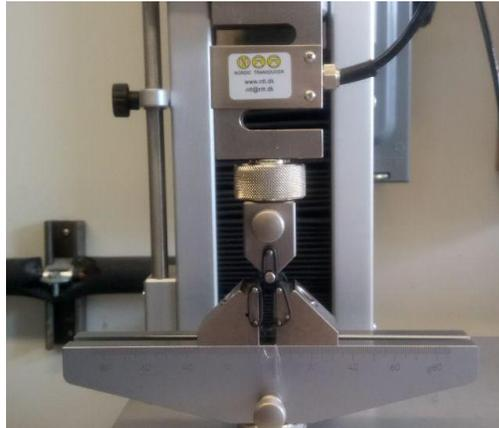
Figure 3: Short Beam Shear (SBS) test setup for short flat beams
