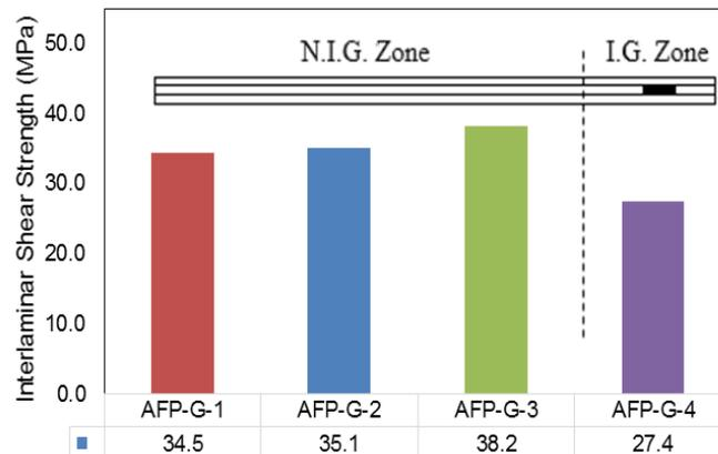
Figure 5: Comparison of the ILSS of the AFP-G samples in I.G. and N.I.G. zones
