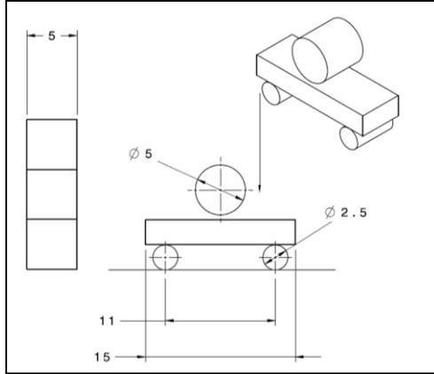
Figure 2: Dimensions of the samples and applied boundary condition for the SBS test
