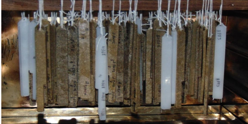
Fig 2: Placement of specimens in hot air oven.
