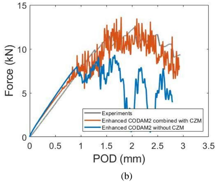
Figure 2 Comparison of the numerical and experimental force vs POD in OCT tests on NCF laminates: (a)  $[90_3/30/-30]_{3s}$  (b)  $[0_3/60/-60]_{3s}$
