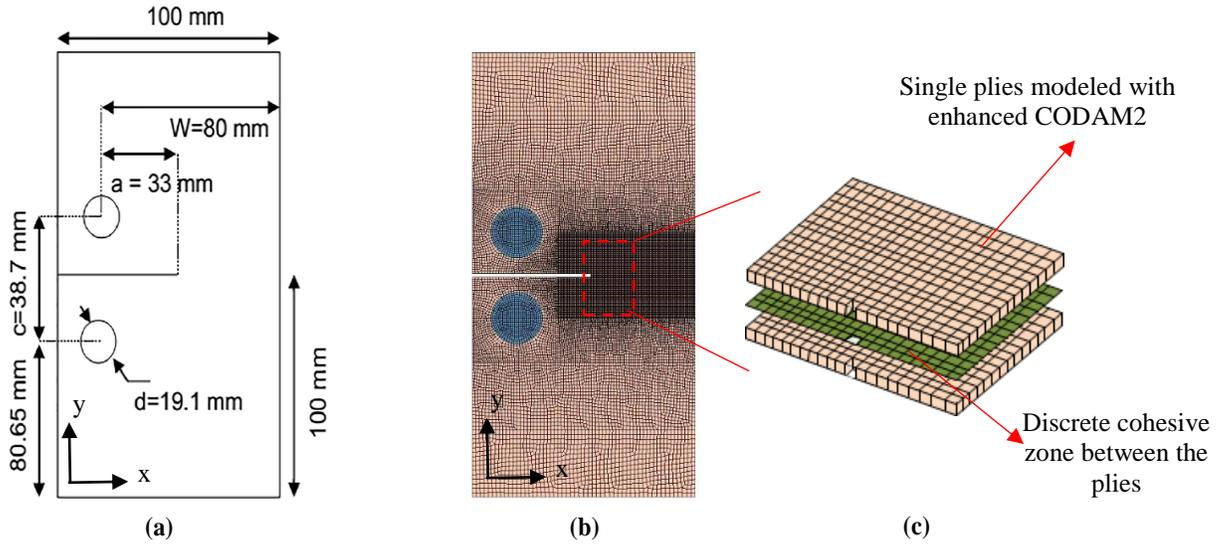
Figure 1: (a) OCT geometry and dimensions, (b) FE mesh for the OCT coupon, (c) Exploded through-thickness view of the region close to the notch tip of OCT specimen showing contact interface between adjacent dissimilar plies (Shahbazi, 2017)
