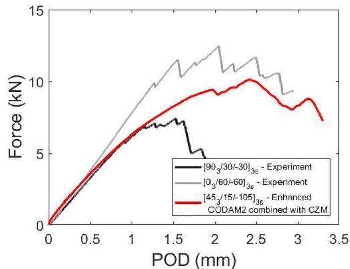
Figure 3 Numerical prediction of the force vs POD curve for  $[45_3/15/-105]_{3s}$  layup superposed on the experimentally obtained curves in the two principal directions
