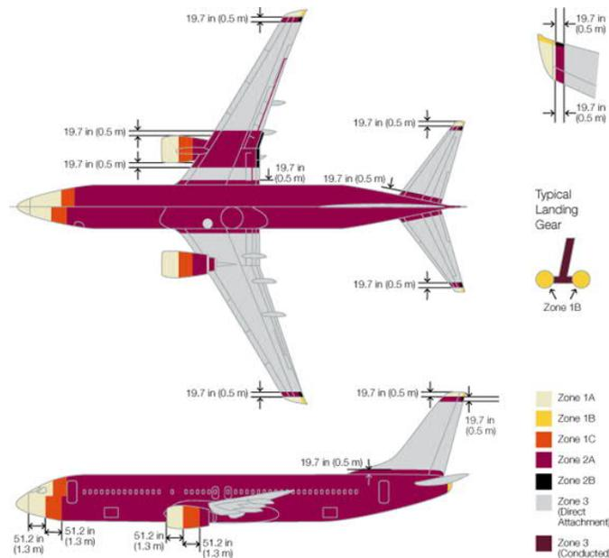
Figure 1: Depiction of lightning zones on a commercial aircraft (SAE Aerospace, 2012)
