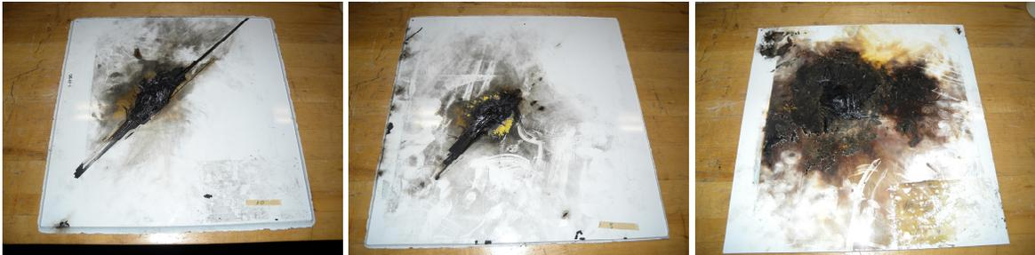
Figure 2: Photos of lightning damage in panels with LSP A, LSP B, and LSP G
