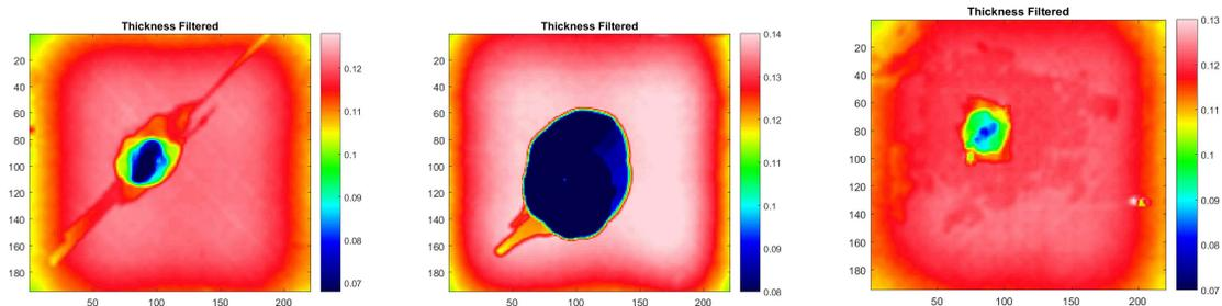
Figure 3: Damage depth in inches for LSP A, LSP B, and LSP G obtained by ultrasonic measurements
