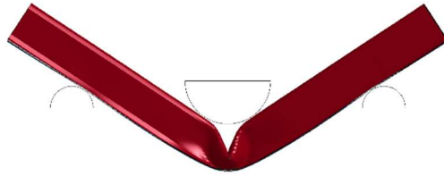
Figure 3: The deformed shape of hybrid beams made of AA7075-T6 and [\pm 45]_s CFRP laminate at the displacement of 135 mm
