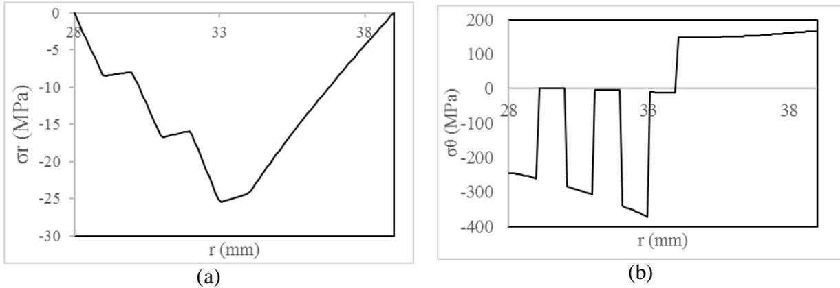
Figure 3: The distribution of a) inter-laminar radial stress b) circumferential stress, through the thickness of the tube 1 at  $\theta = 90^\circ$ , at first ply failure based on Tsai-Wu criterion ( $M_x=17.3$  KN.m.).
