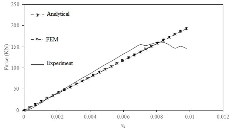
Figure 6: Change of longitudinal strain (mid-length and bottom surface) with applied force for three-point bending of tube 2,  $[90_{30}^{\circ} / \pm 25_{45}^{\circ} / 90_5^{\circ} / \pm 30_{20}^{\circ} / 90_5^{\circ} / \pm 45_{20}^{\circ}]$ .
