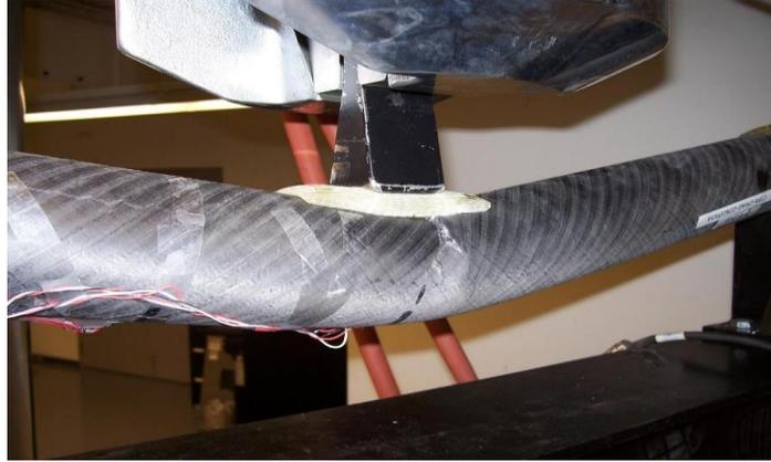
Figure 5: Fracture of tube 1 due to stress concentration at the loading nose, (Derisi 2008).
