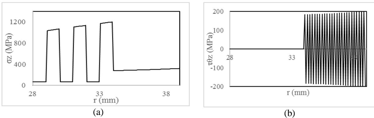
Figure 4: The distribution of a) the longitudinal stress b) the out-of-plane shear stress through the thickness of the tube 2 at  $\theta = 90^\circ$ , at first ply failure based on Tsai-Wu criterion ( $M_x=17.3$  KN.m.).
