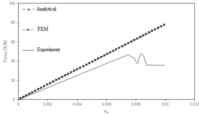
Figure 2: Change of longitudinal strain (mid-length and bottom surface) with applied force for three-point bending of tube 1,  $[(90_{10}^{\circ} / 0_{10}^{\circ})_3 / \pm 45_{25}^{\circ}]$ .
