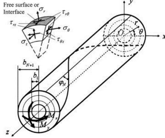
Figure 1: A composite tube subjected to pure bending (Zhang et al. 2014).
