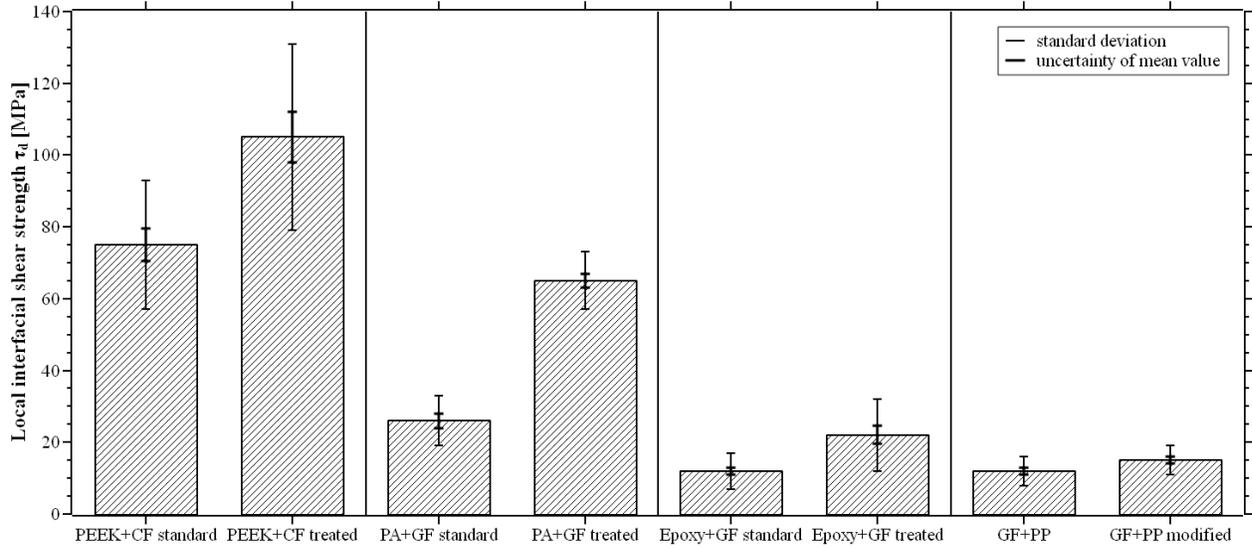
Figure 7: Local interfacial shear strength  $\tau_d$  of standard and treated fibers in different matrices. The bars indicate the mean value found in 15 trials. The error bars show the standard deviation and the uncertainty of the mean value.
