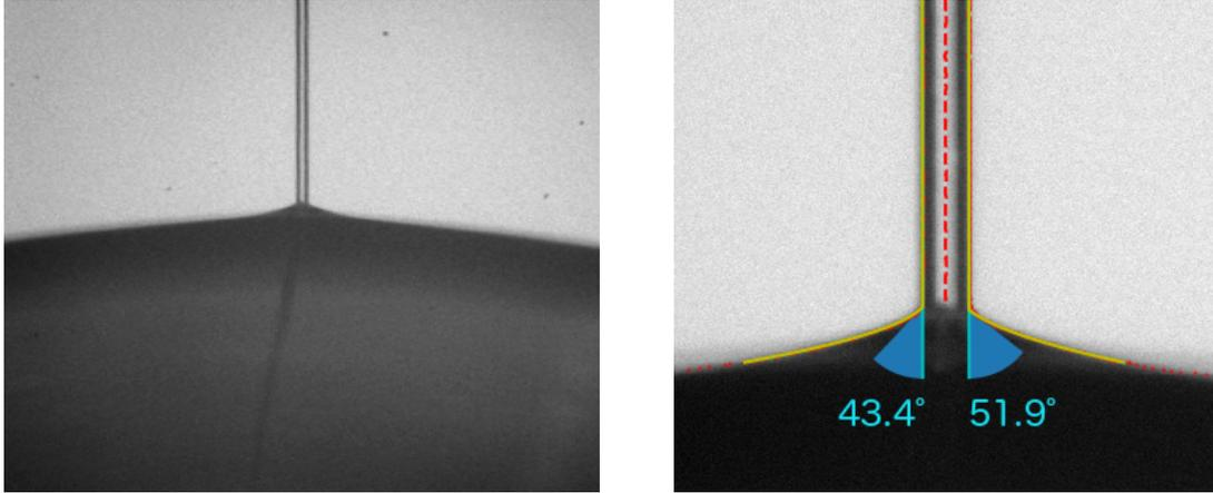
Figure 4: Observation of the meniscus forming between fibre and matrix during the embedding process as seen by the FIMABOND device – here, between a glass fibre and an epoxy resin. Left: the full image, right: the automatic evaluation of the contact angle on both sides of the fiber.
