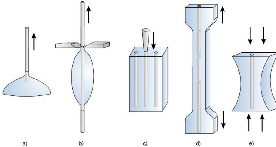
Figure 1: Overview of micromechanical tests methods for measuring the fiber-matrix adhesion: pull-out (a), microbond (b), push-out (c), fragmentation (d) and Broutman (e) (Mäder et al., 2016).
