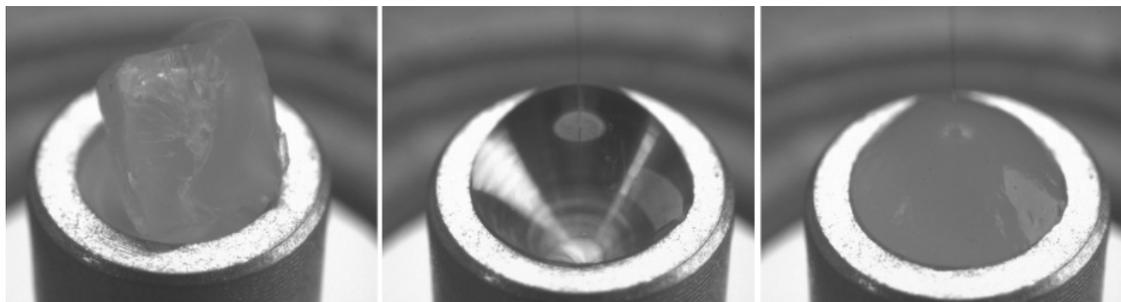
Figure 3: Process of embedding a glass fiber into PA 6 with the FIMABOND, left: flushing sample with inert gas, center: melting of the matrix material and contact between the fiber and the matrix surface and embedding, right: cooling and consolidation of the sample
