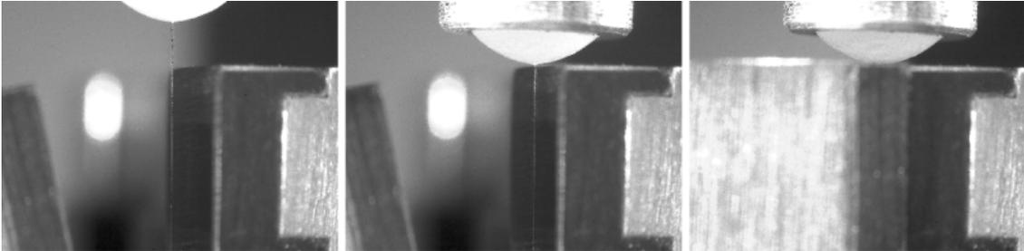
Figure 5: Process of adjusting the sample in the clamping system. The sample is placed with the fiber pointing down and held by the force transducer of the FAVIMAT+ testing machine (left). The fibre is aligned parallel to the right-hand side yaw face (mid) and clamped at minimal distance to the matrix droplet (right).
