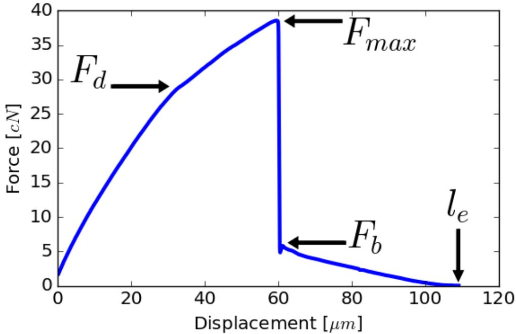
Figure 6: Force-displacement curve of glass fiber and epoxy resin.
