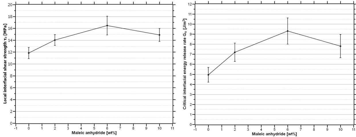
Figure 8: Fibre-matrix adhesion strength between GF and PP as a function of wt% maleic anhydride masterbatch in the PP. The error bars indicate the uncertainty of the mean value using 15 trials. Left: strain-based evaluation applied to the pull-out data, right: the energy-based evaluation is used. In both cases the maximum adhesion is found at 6 wt% masterbatch.
