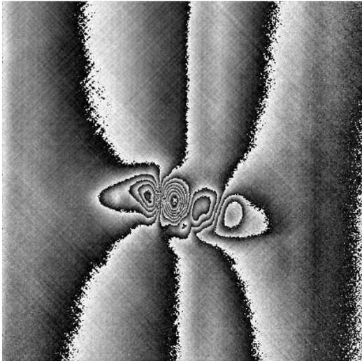
**Figure 8 Thermal Wrapped Shearography image of non-visible impact to a solid laminate wing panel**
