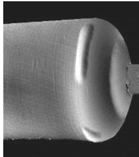
**Figure 11 Shearography image of the end of a 6.3 inch diameter COPV showing fiber bridging on the barrel transition area.**
