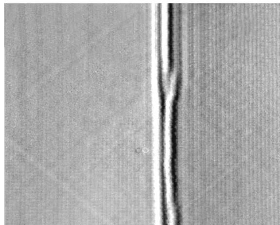
**Figure 7 Wrinkled fiber in carbon fiber laminate imaged with thermal shearography.**
