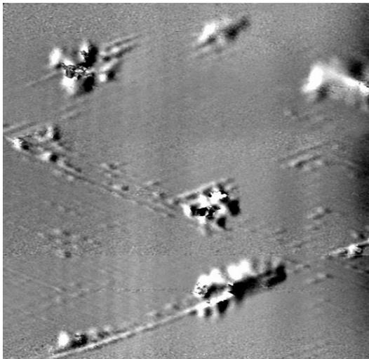
**Figure 10 Pressure Shearography image of a composite tube showing porosity, voids, and poor consolidation**
