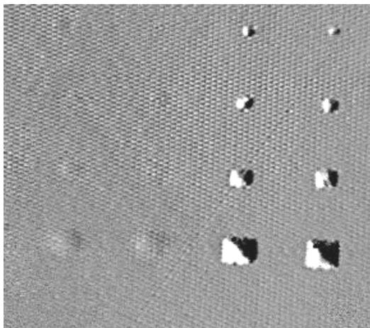
**Figure 6 Spacecraft reflector NDT STD tested with thermal shearography showing disbands.**
