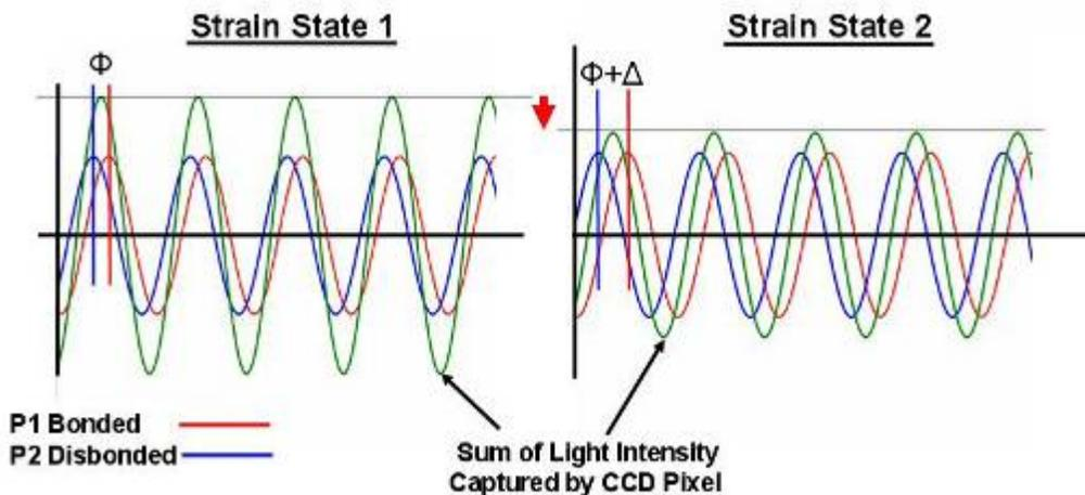
**Figure 2 Change in signal intensity due to phase shift with a change in strain state.**
