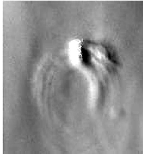
**Figure 9 Thermal Shearography image of an eight inch diameter composite repair on an aircraft vertical stabilizer**
