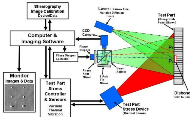
**Figure 1 Schematic Diagram of a digital shearography camera and thermal stress system.**
