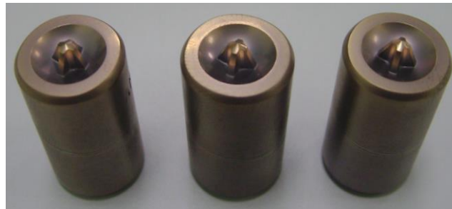
Figure 5. CrAlTiSiN-coated Phillips punches.
