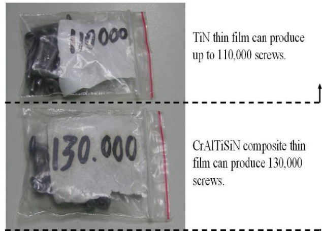
Figure 7. A comparison of the number of extrusion forgings for Philips screws using various coated punches.
