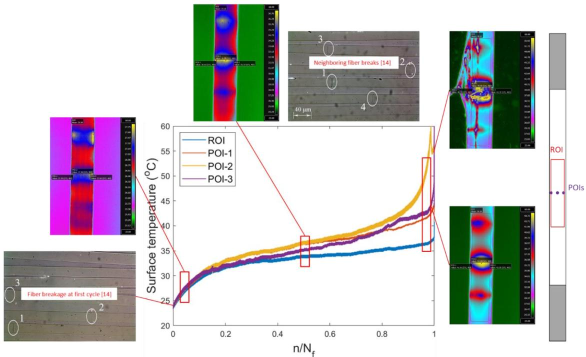
Figure 6. Surface temperature evolution for RT fatigue specimens with peak stress of 65% UTS
