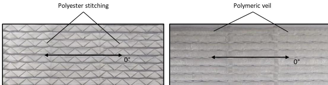
Figure 1. Photograph of UD-NCF glass fabric (a) upper surface with tricot stitching patterns, and (b) bottom surface with veil
