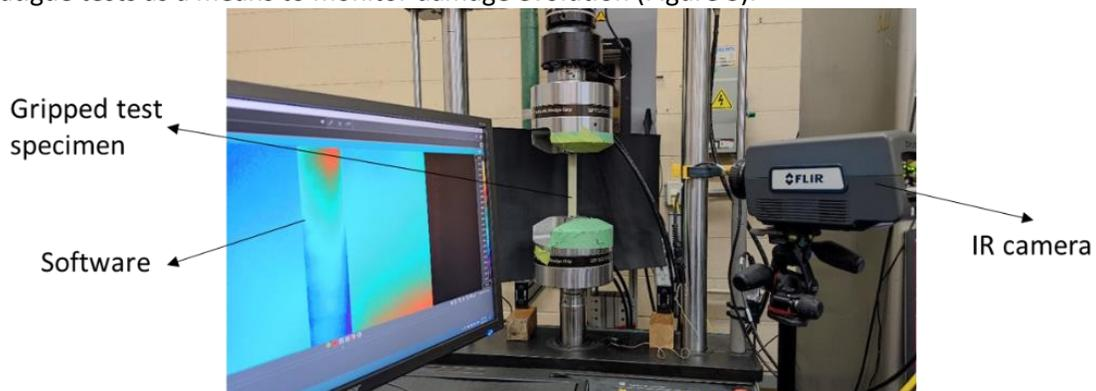
Figure 3. RT fatigue test set-up with IR camera
