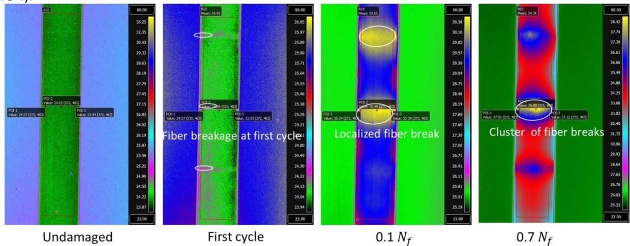
Figure 8. Damage evolution for RT fatigue tests under a peak stress of 65% UTS
