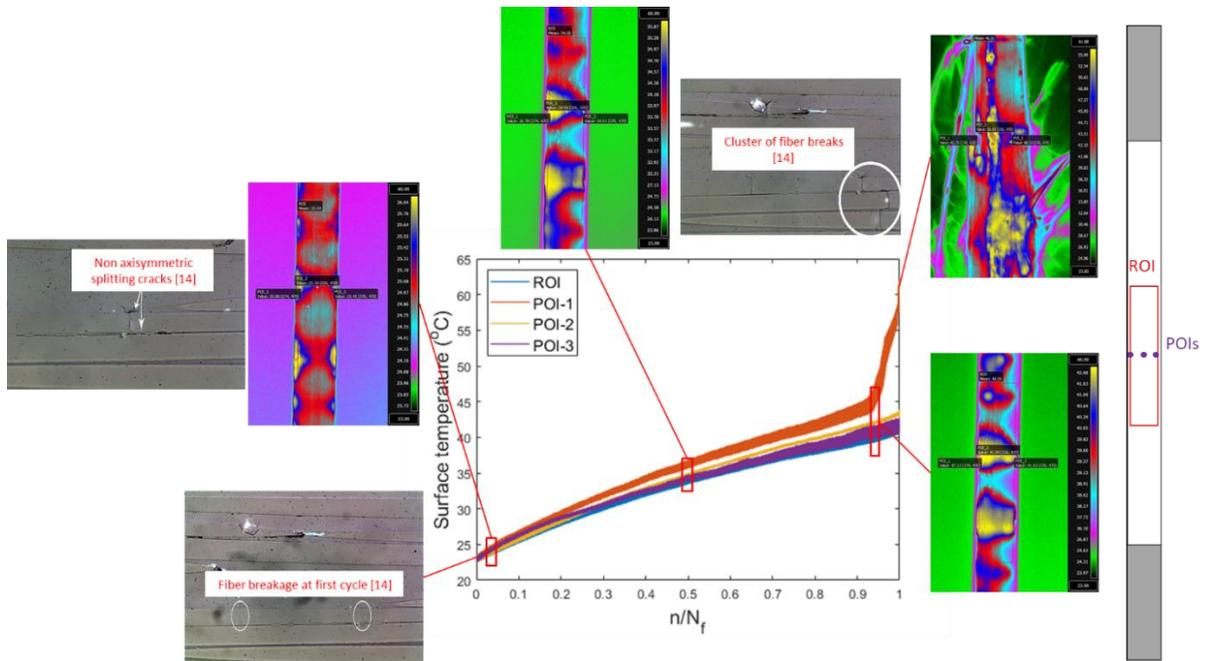
Figure 5. Surface temperature evolution for RT fatigue specimens with peak stress of 85% UTS
