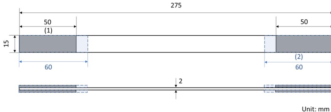
Figure 2. Photograph of specimen geometry for RT (1) and -50°C (2) tests (fibers oriented along the specimen axis).
