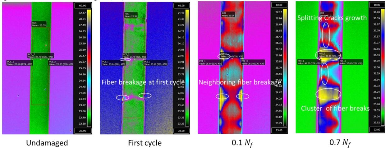
Figure 7. Damage evolution for RT fatigue tests under a peak stress of 85% UTS
