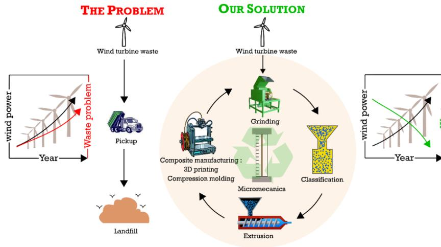
Figure 1. The recycling schemes of mechanical grinding and FFF 3D printing [11].
