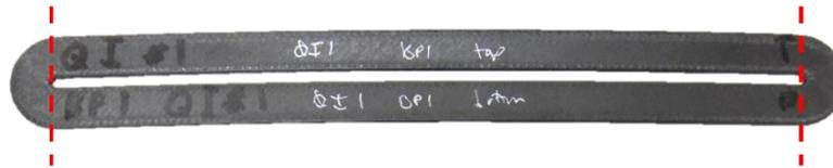
Figure 2: “Racetrack” configuration used to 3D print samples to characterize with and without reinforcement
