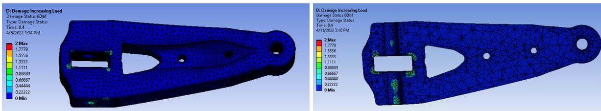
Figure 7. Damage status at 60lbf: full part (left), cross-section (right).
