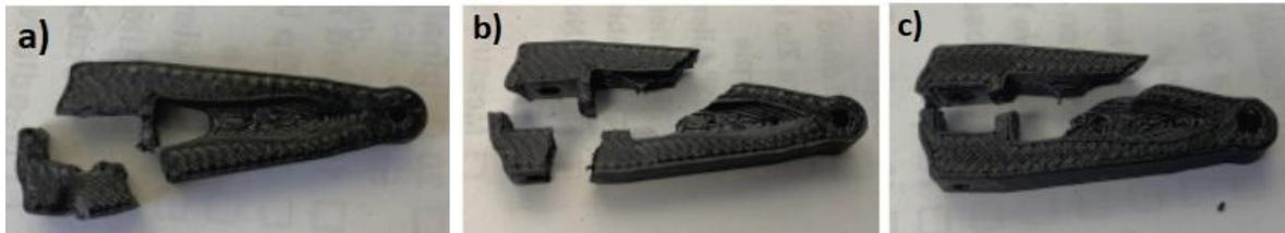
Figure 14. Antero 840CN03 failure locations.
