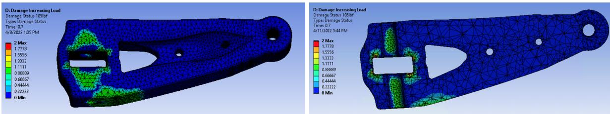
Figure 10. Damage status at 105lbf: full part (left), cross-section (right).
