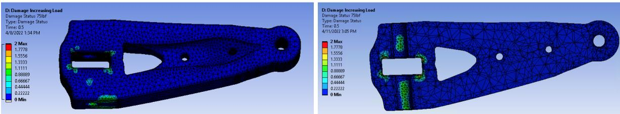
Figure 8. Damage status at 75lbf: full part (left), cross-section (right).
