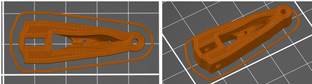
Figure 15: FDM™ tool path for Proposed Lever
