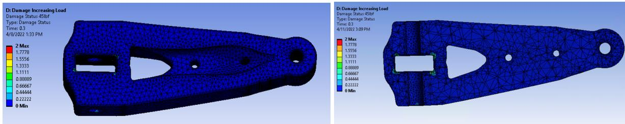
Figure 6. Damage status at 45lbf: full part (left), cross-section (right).
