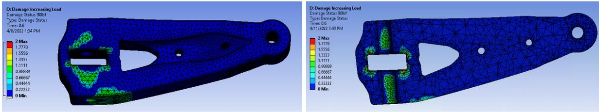
Figure 9. Damage status at 90lbf: full part (left), cross-section (right).
