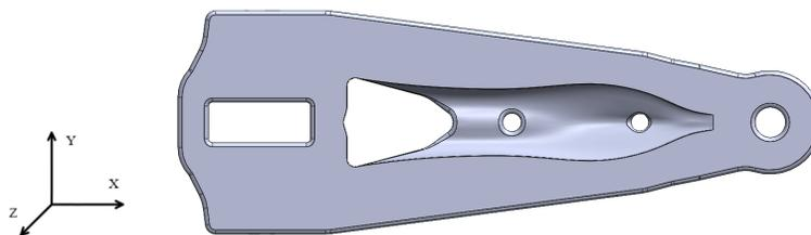
Figure 1. Resulting CAD model of the final lever design.
