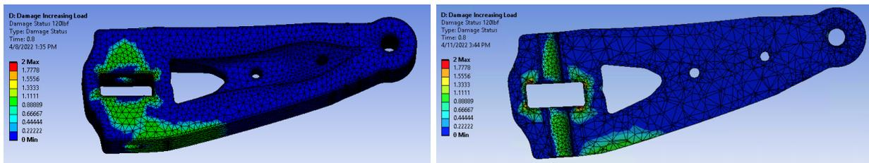
Figure 11. Damage status at 120lbf: full part (left), cross-section (right).
