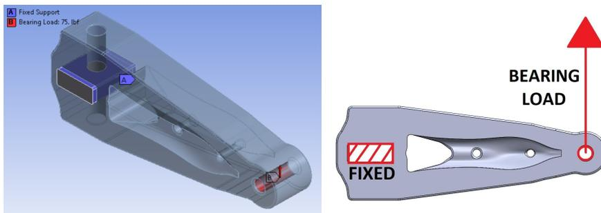
Figure 2. Fixed support and bearing load.
