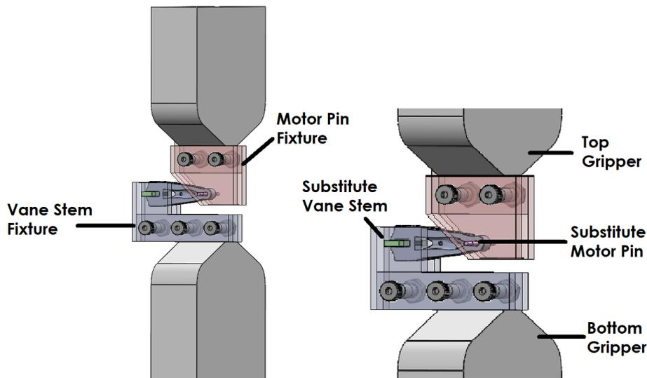
Figure 4. Testing rig assembly.
