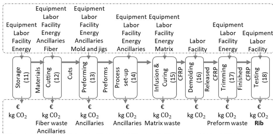
Figure 4. Manufacturing process model for scenario (2): hand lay-up and autoclave.
