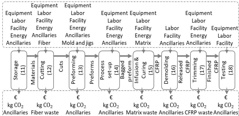
Figure 3. Manufacturing process model for scenario (1): hand lay-up, single-line infusion, and autoclave.
