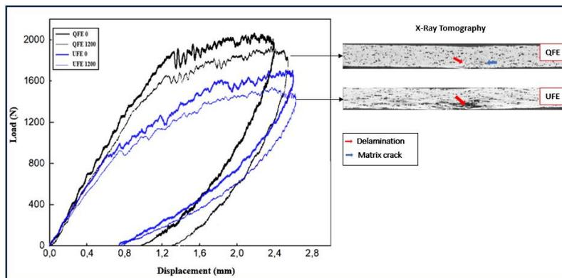
Figure 5. Drop-Weight-Impact and X-ray Tomography of the QFE and UFE configurations.
