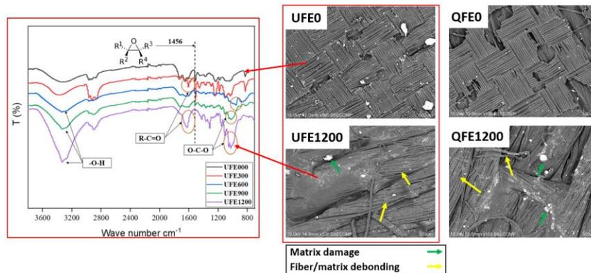
Figure 3. FTIR and SEM images of the UFE and QFE samples before and after 1200 h of weathering time.
