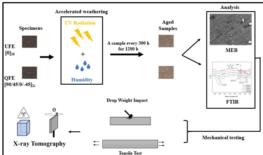
Figure 1. Experimental procedure.
