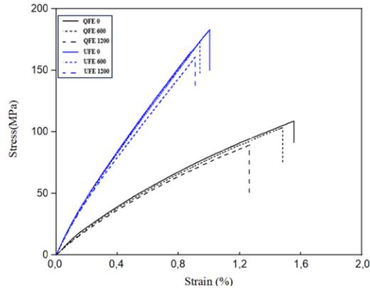
Figure 4. Stress-Strain curves for the UFE and QFE configurations at 0, 600 and 1200 h of weathering time.
