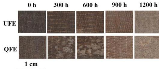
Figure 2. Color change as function of weathering time.
