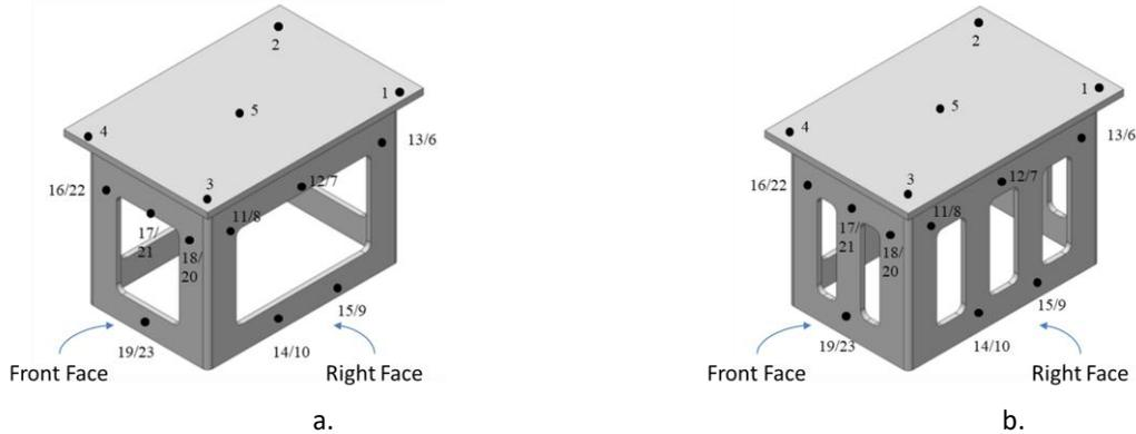
Figure 2. Thermocouple locations on the open mould (a) and closed mould (b) tools. At any location x/y denotes TC<sub>x</sub> is located on the visible face and TC<sub>y</sub> is located on the opposite face not visible on the images
