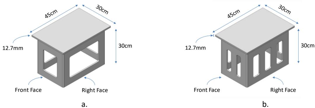
Figure 1. Schematic of the (a) open and (b) closed substructure steel tools used in this work
