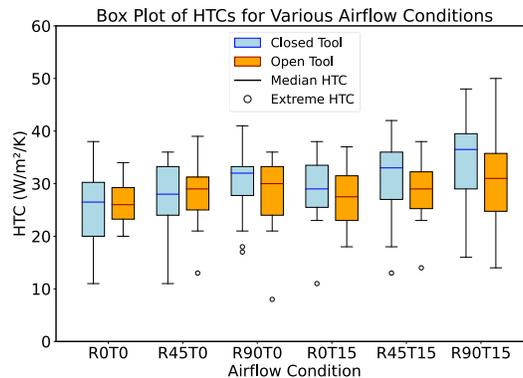
Figure 5. Box plot showing HTC's for both the tools for different airflow conditions
