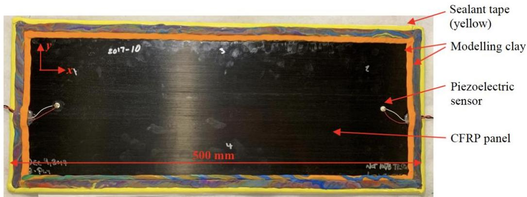
Figure 1. CFRP panel with piezoelectric sensors [2].
