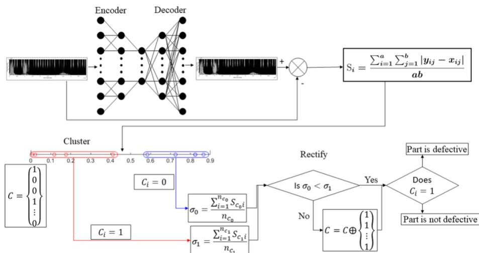
Figure 5. Schematic of the proposed analysis methodology.
