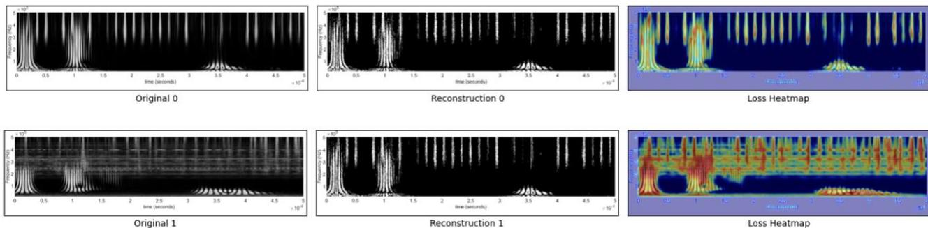
Figure 6. Example of panels which were correctly classified by the proposed method. The numbers “0” and “1” represent a non-defective and defective panel respectively. The damaged panel was known to have a delamination defect under the second ply.
