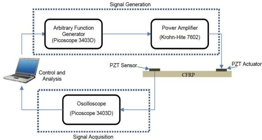
Figure 2. Experimental setup to generate and collect Lamb wave signals [2].
