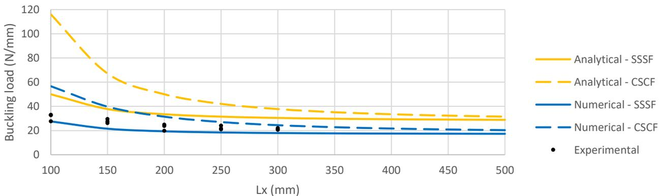
Figure 3 Experimental, analytical, and numerical buckling load for a 15 plies cardboard angle with  $L_y = 50$  mm.
