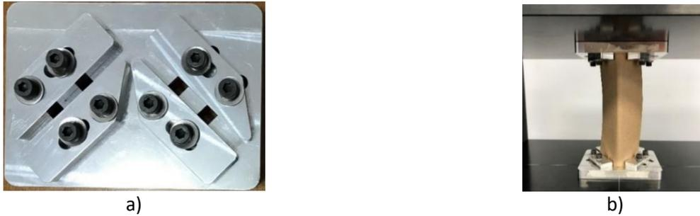
Figure 1 Experimental set-up: a) custom adjustable device and b) angle mounted assembly.
