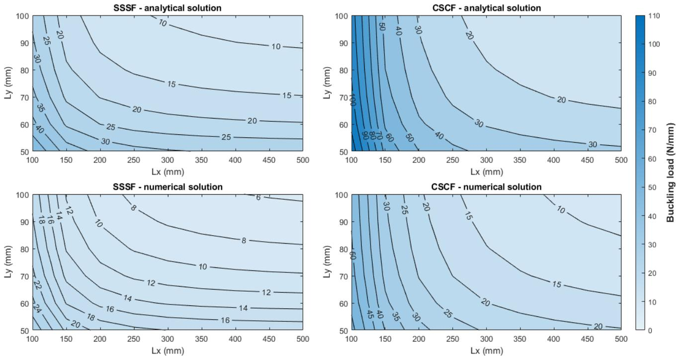
Figure 2 Buckling load for a 15 plies laminate obtained by analytical and numerical study for SSSF and CSCF boundary conditions.
