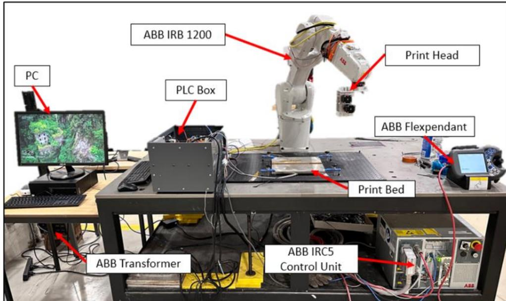
Figure 1. The robotic 3D printing set-up.
