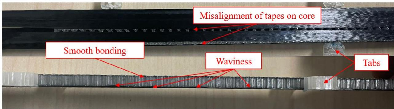
Figure 5. Visual observations of drum peel test specimen before testing.
