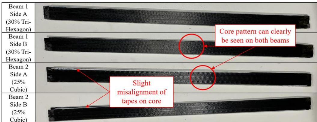
Figure 2. Co-consolidation robotic 3D printed thermoplastic sandwich specimens side observations.
