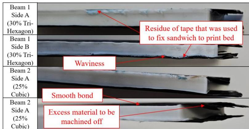
Figure 3. Co-consolidation robotic 3D printed thermoplastic sandwich specimens cross section observations.
