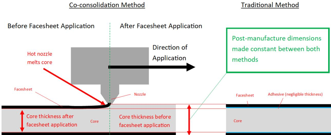
Figure 4. Co-consolidation versus traditional method core thicknesses considerations.
