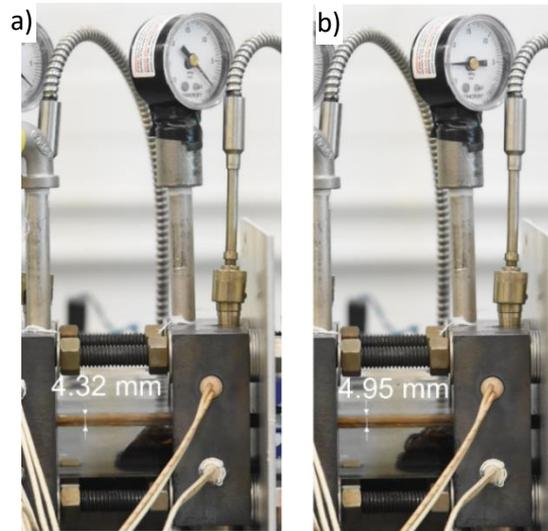
Figure 2. View of the pultrudate in between dies through the quartz vacuum chamber with a)  $P_{atm}$  and b) partial vacuum.
