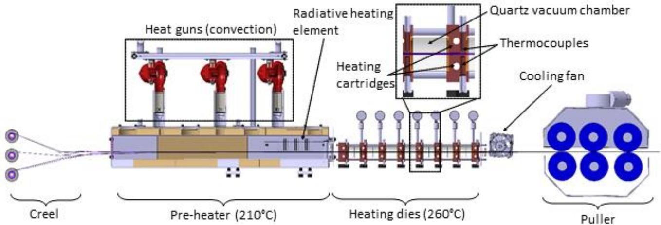
Figure 1. Schematic view of the multi-die pultrusion line.
