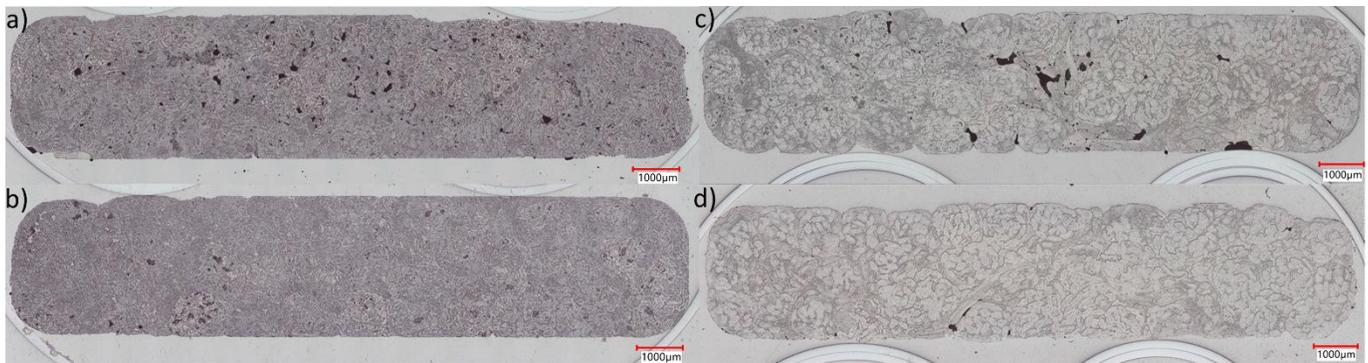
Figure 3. Micrographs of pultruded specimens at 100 mm/min a)  $P_{atm}$  b) vacuum, and at 500 mm/min c)  $P_{atm}$  d) vacuum. The fibers are shown in white, the matrix in gray, and the dark areas are voids.
