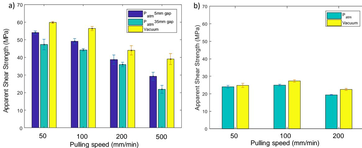
Figure 4. Short-beam strength of a) GF/PA6 specimens and b) GF/PP pultruded at different speeds and pressure conditions.
