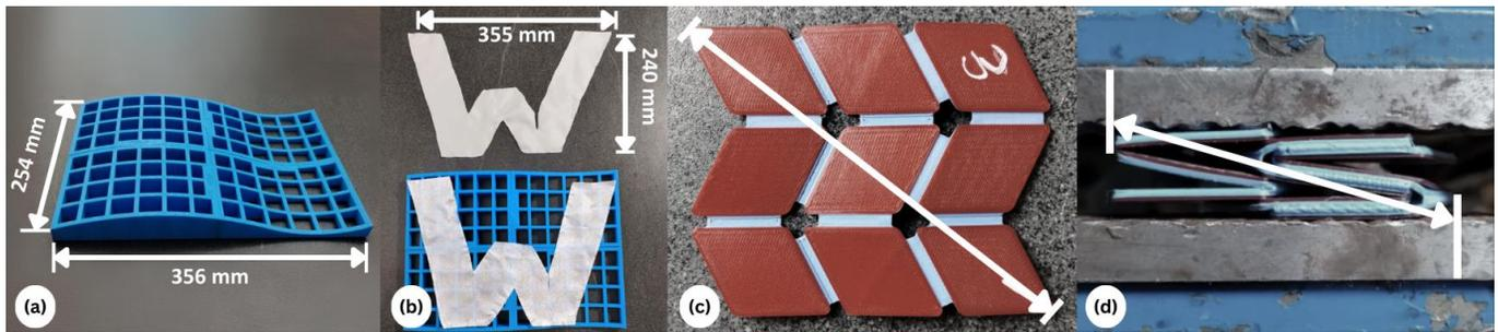
Figure 1. (a) the mould, (b) the W shape, (c) open gripper distance and (d) compressed/closed gripper distance.
