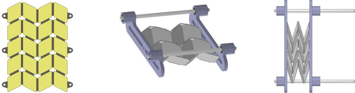
Figure 3. (a) sample gripper with frame connections (loops) (b) partially and (c) fully compressed frame and gripper (with the linear rod and bearing).
