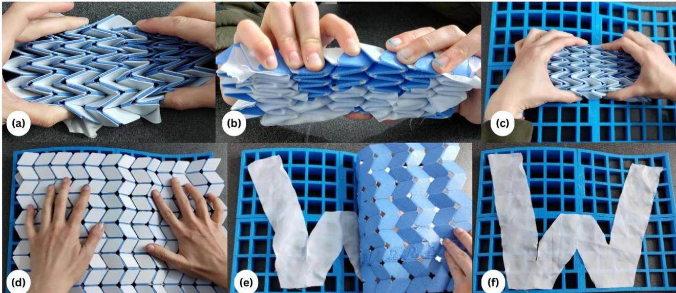
Figure 2. Manual pick and place testing including (a) pick, (b)(c) transfer, and (d)(e)(f) place.
