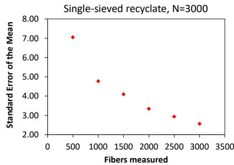
Figure 7. Standard error of the mean for single-sieved fine recycle.
