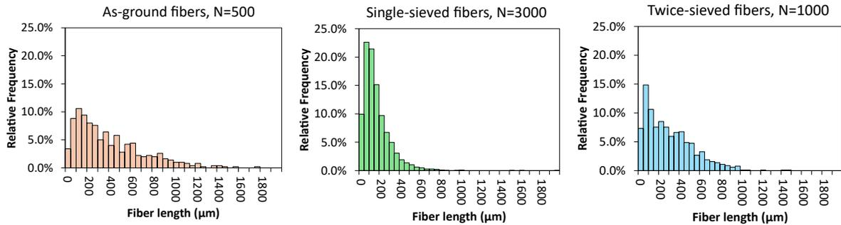
Figure 6. Fiber length distributions for a) as-ground fibers, b) single-sieved fibers, and c) double-sieved fibers.
