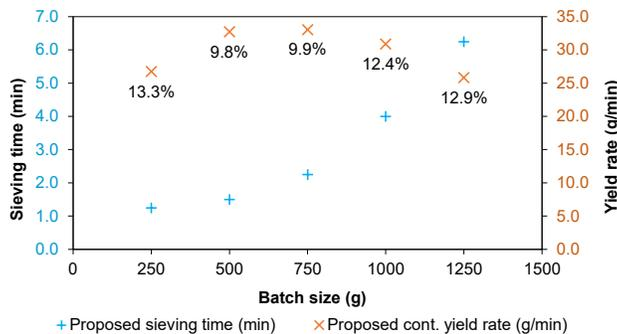
Figure 3. Addition of average yield rate onto Figure 2c. The proposed batch size for the given setup is 500-750g while the corresponding optimal sieving times were around 1.5-2 minutes.
