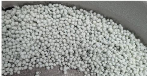
Figure 5. Agglomeration of recyclate during repeated sieving. A mix of long and short fibers can be seen in each clump.
