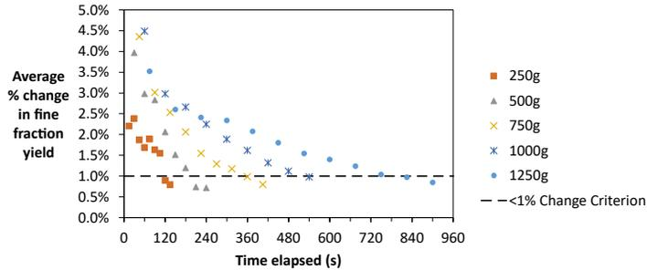
Figure 1. Total sieving time required given <1% change stopping criterion for input masses 250g to 1250g in 250g intervals.
