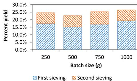
Figure 4. Total fine recyclate yield at the <1% change criterion following a double-sieving process ( $N \leq 2$  repeats). 1250g was omitted due to lack of data.
