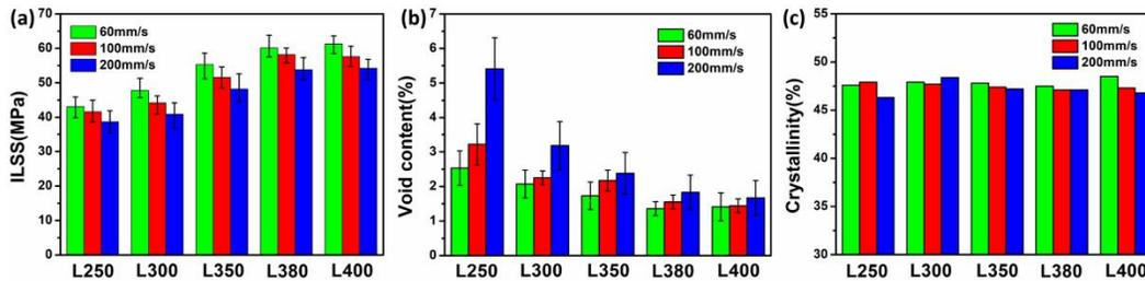
Figure 5. ILSS (a), void content (b) and crystallinity (c) of  $[0]_{20}$ CF/PPS laminates with different parameters.
