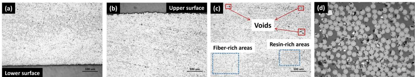
Figure 4. Cross-sectional morphology of laminate 1#. (a: lower surface; b: upper surface; c-d: different magnification)
