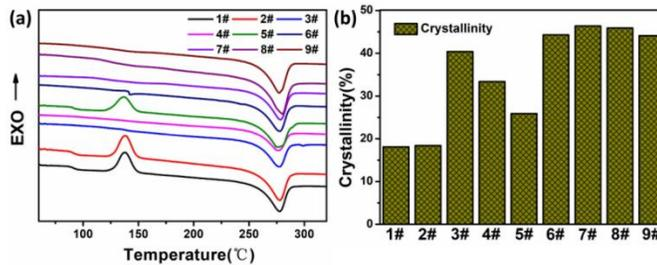
Figure 3. DSC curves (a) and related crystallinity (b) of all laminates.
