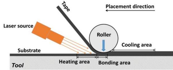
Figure 1. Schematic illustration of laser-assisted AFP in-situ consolidation process of thermoplastic composites.
