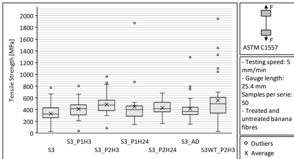
Figure 2: Tensile strength of treated and untreated BFs (only outlier points are shown)
