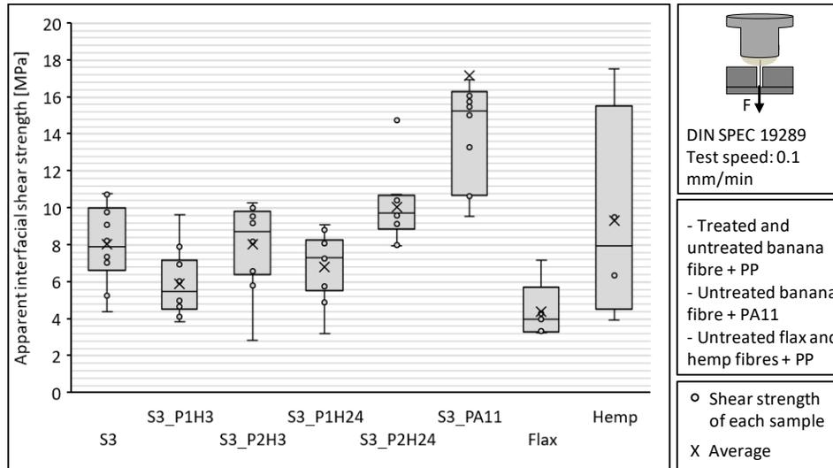
Figure 3: Apparent interfacial shear strengths ( $\tau_{app}$ ) of BFs embedded in PP; S3\_PA11, Flax and hemp as references
