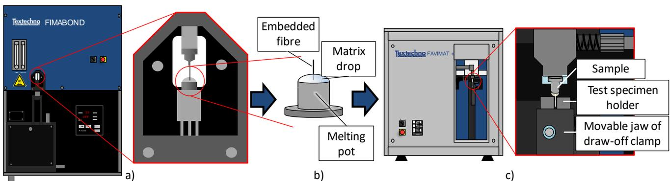
Figure 1: a) Pull-out sample preparation machine FIMABOND; b) Pull-out test sample; c) Pull-out testing machine, FAVIMAT
