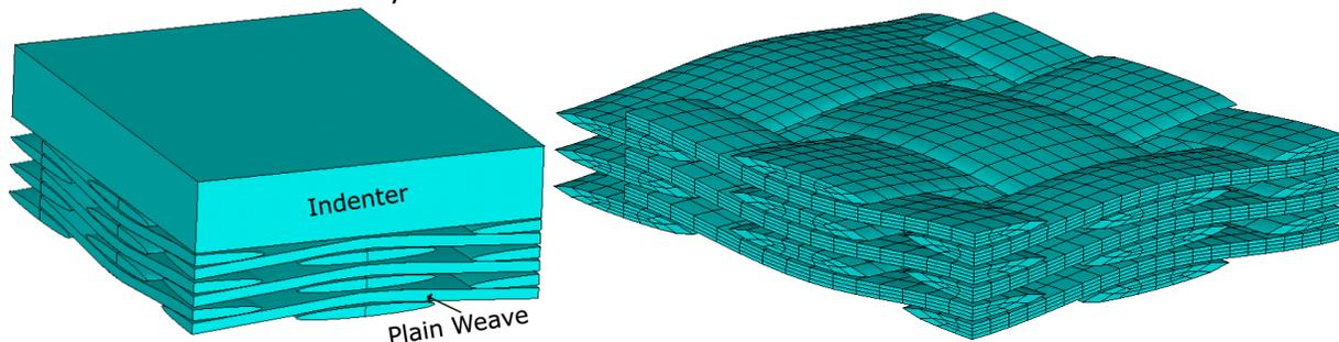
Figure 2: (Left) Solid model of the RVE with a section of indenter. (Right) Mesh of the RVE.
