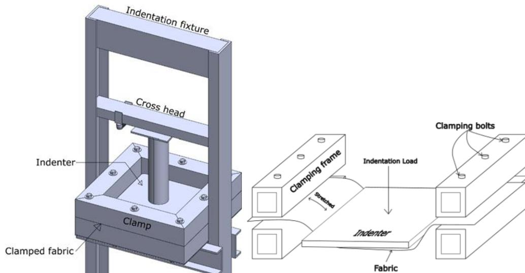
Figure 1: (Left) Indentation Fixture components. (Right) Mechanism of applying 1-D prestress.
