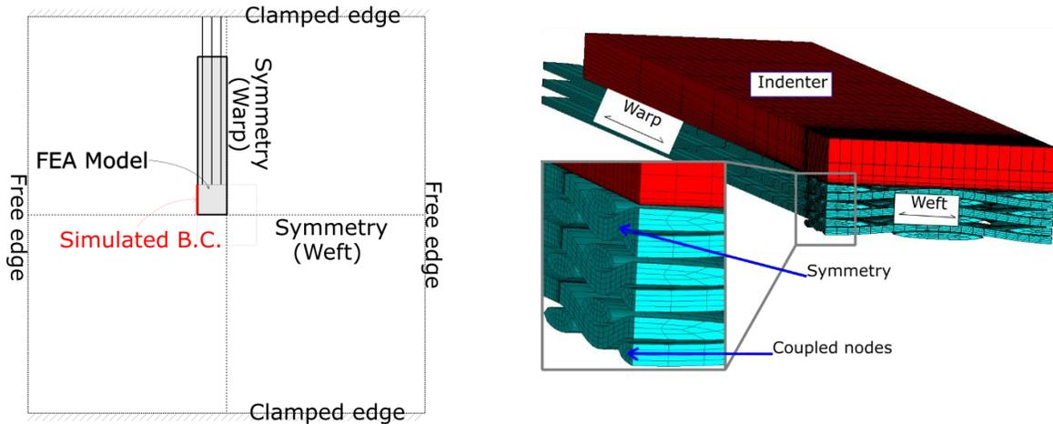
Figure 3: (Left) The RVE position on the fabric. (Right) The mesh of the RVE, its extended warp yarns, and the indenter with Simulated B.C.
