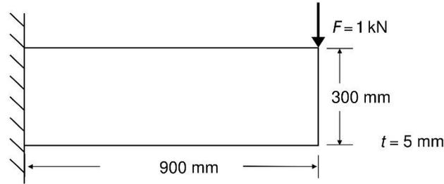
Figure 2. Load and boundary conditions of a cantilever beam.
