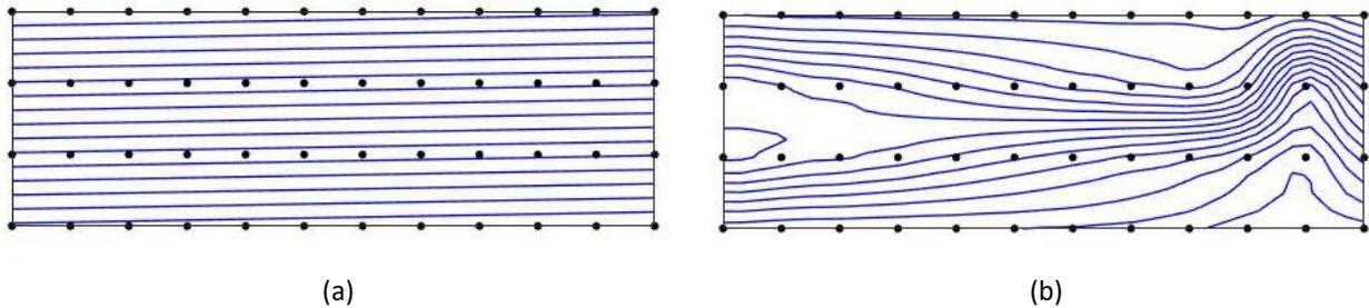
Figure 3. The optimization result of a cantilever beam after 306 iterations (50 seconds). (a) is the initial fibre pattern with  $1^\circ$  fibres, and (b) is the optimized contour with compliance reduced by 19%. The blue lines are fibre contours, and black dots are the locations of RBF centres.
