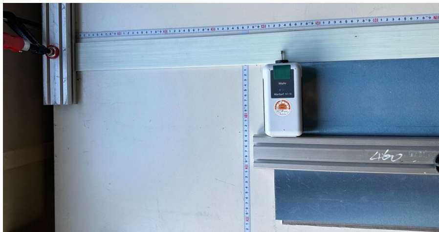
Figure 9. Setup of the surface roughness measurement device (top view). Measurement taken perpendicular to pulling direction.
