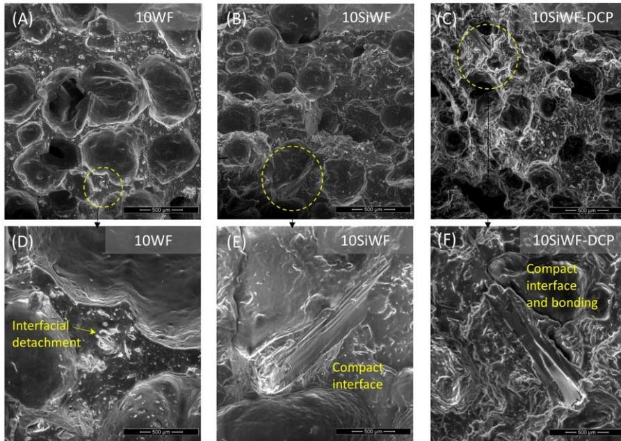
Figure 2. Cell and fiber morphology of the EPDM foam filled with wood fiber.
