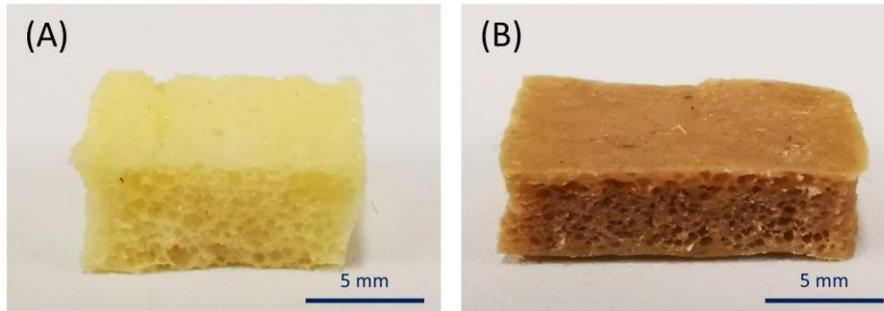
Figure 1. Real life EPDM foams. (A) Pure foam; (B) 10SiWF-DCP
