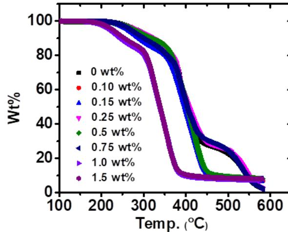
Figure 2. Thermal degradation behavior of epoxy CNWs nanocomposites observed from TGA analysis.
