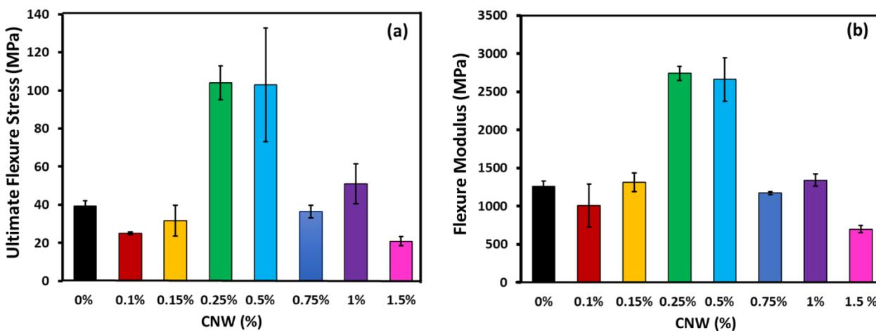
Figure 3. Flexure load behavior of epoxy CNWs nanocomposites: (a) Ultimate flexure stress and (b) Flexure modulus.
