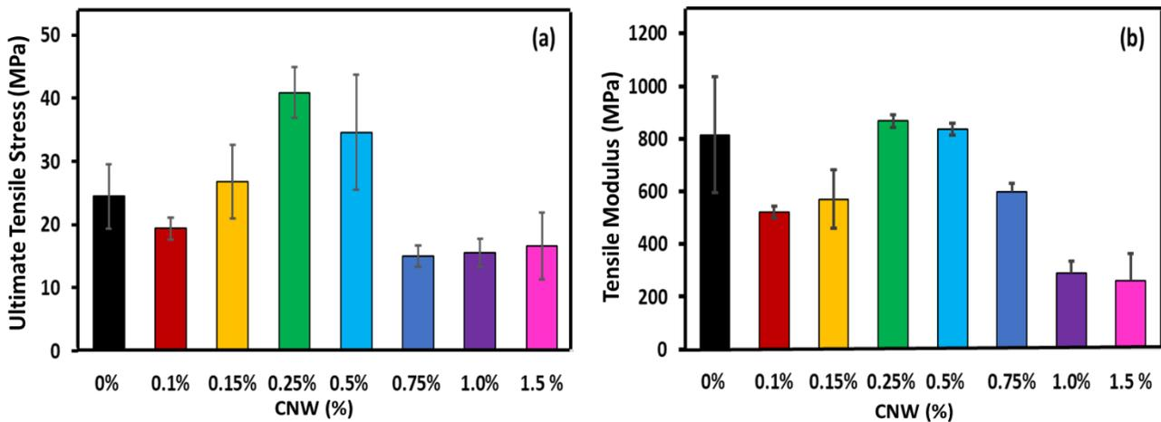
Figure 4. Tensile characteristics of epoxy CNWs nanocomposites: (a) Ultimate tensile stress and (b) Tensile modulus.
