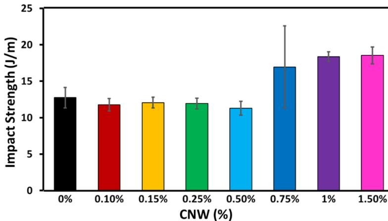
Figure 5. IZOD Impact strength of the epoxy CNWs nanocomposites.
