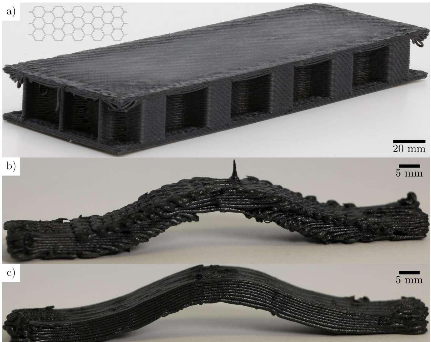
Figure 3 – CF-PEEK printed part of a) a full sandwich panel with a length of 212 mm and a honeycomb core, b) a curved beam printed with a planar toolpath and c) the same curved beam geometry printed following a non-planar toolpath.
